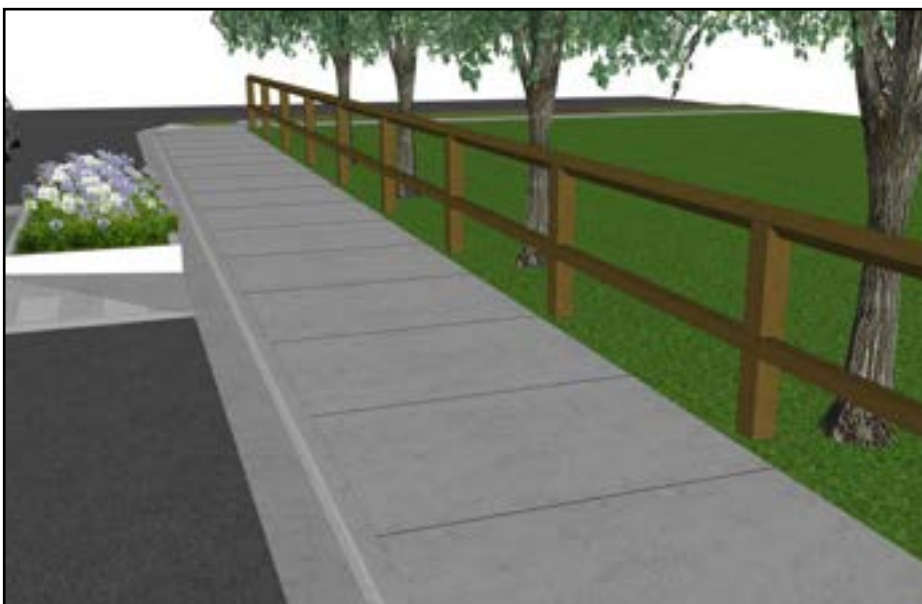
1.5m wide concrete footpath
