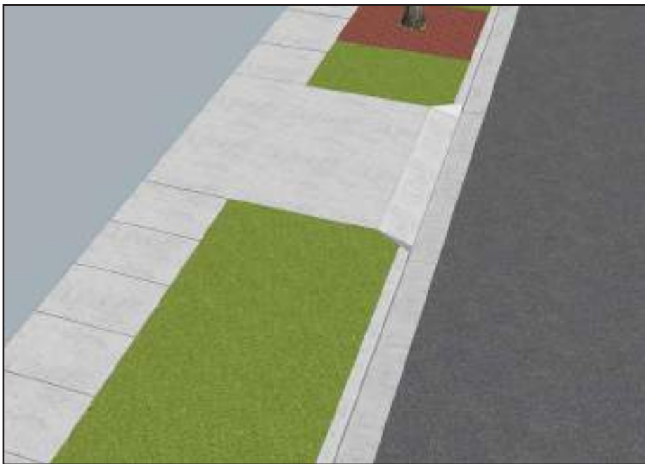
1.5m wide concrete footpath
