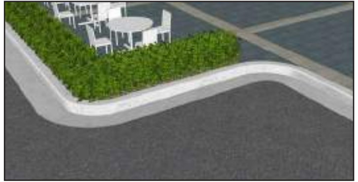
Kerb and gutter treatment
