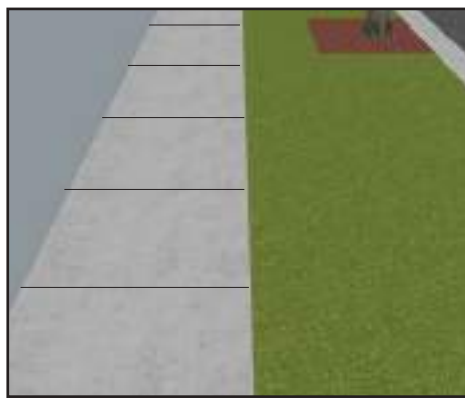
1.5m wide concrete footpath
