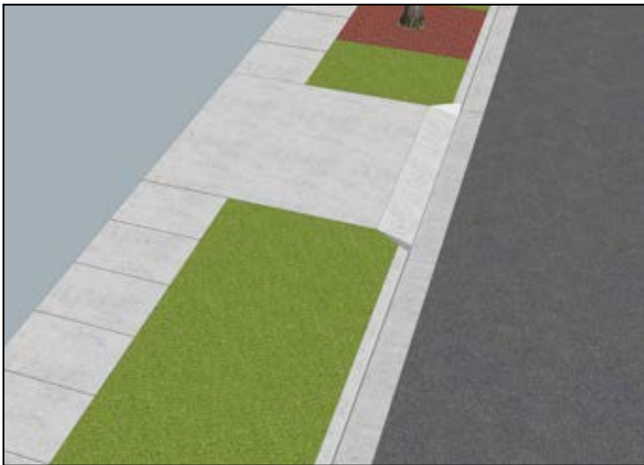
1.5m wide concrete footpath
