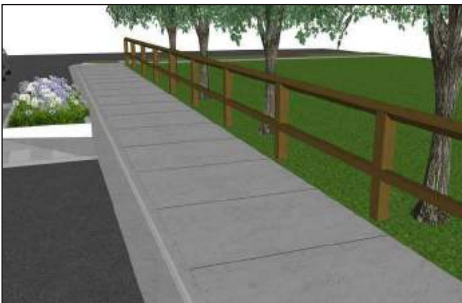
1.5m wide concrete footpath
