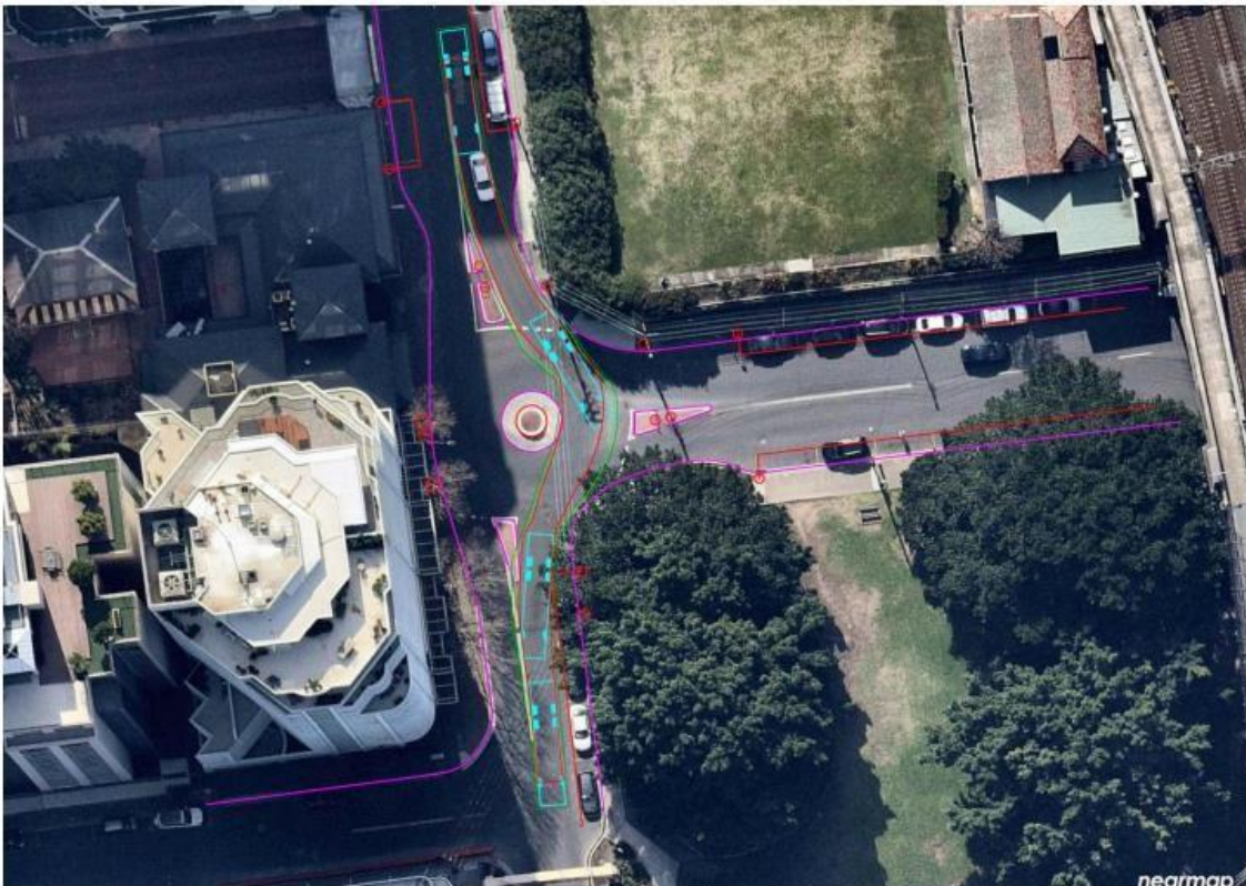
4 Alfred Street, Milsons Point Swept Path Diagram Alfred Street South, Continue onto Alfred Street South (Southbound) 12.5 x 2.5m Heavy Rigid Vehicle (0.3m Clearance) Scale 1:500 @ A4 Plan Prepared by Jim's Traffic Control (Hornsby) Date 23/02/2021
