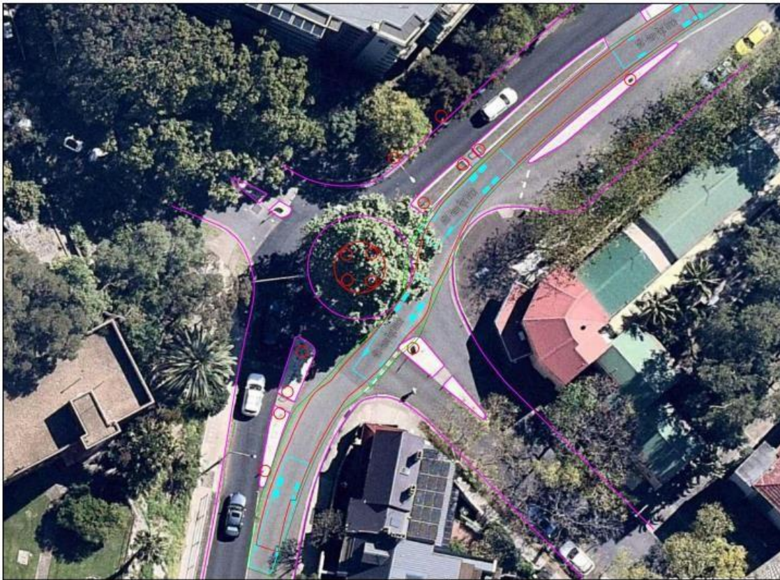
4 Alfred Street, Milsons Point Swept Path Diagram Clark Road, Continue onto Broughton Street 12.5 x 2.5m Heavy Rigid Vehicle (0.3m Clearance) Scale 1:500 @ A4 Plan Prepared by Jim's Traffic Control (Hornsby) Date 23/02/2021 Sheet 12
