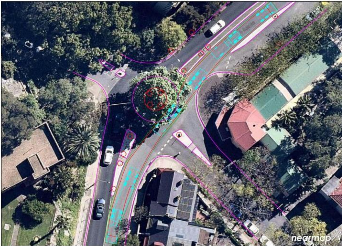
4 Alfred Street, Milsons Point Swept Path Diagram Clark Road, Continue onto Broughton Street 19 x 2.5m Articulated Vehicle (0.3m Clearance) Scale 1:500 @ A4 Plan Prepared by Jim's Traffic Control (Hornsby) Date 13/02/2021
