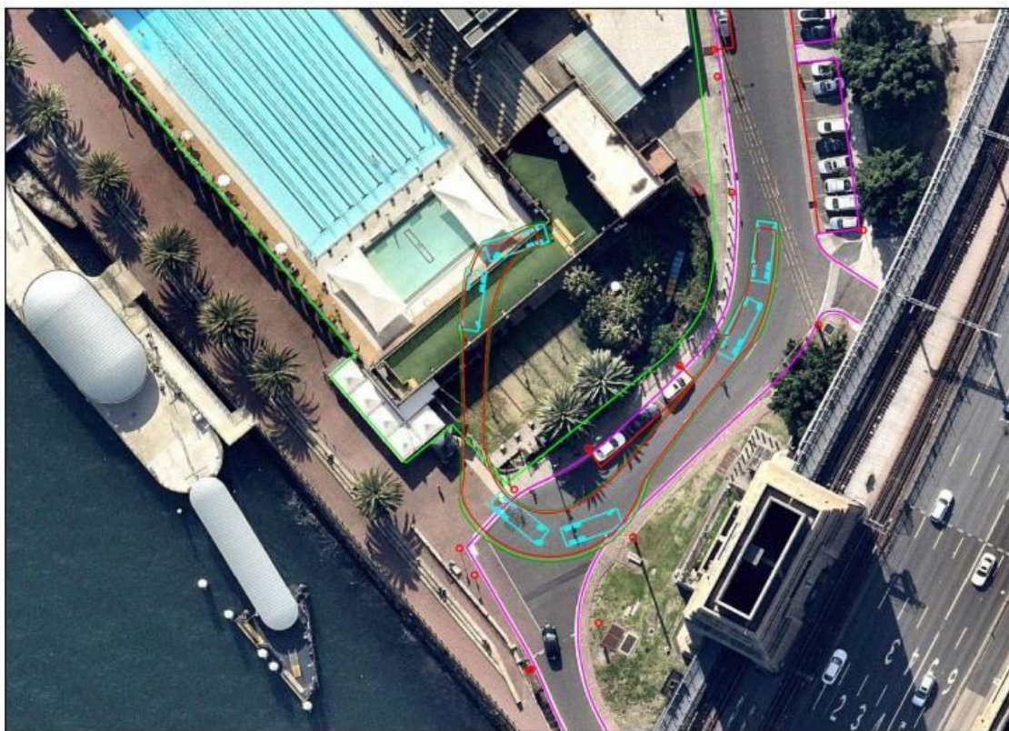
4 Alfred Street, Milsons Point Swept Path Diagram Site (Gate 1), Turn Left onto Alfred Street South
