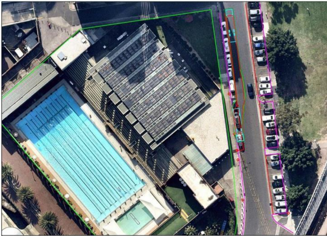
4 Alfred Street, Milsons Point Swept Path Diagram Work Zone, Turn Right onto Alfred Street South 12.5 x 2.5m Heavy Rigid Vehicle (0.3m Clearance) Scale 1:500 @ A4 Plan Prepared by Jim's Traffic Control (Hornsby) Date 23/02/2021
