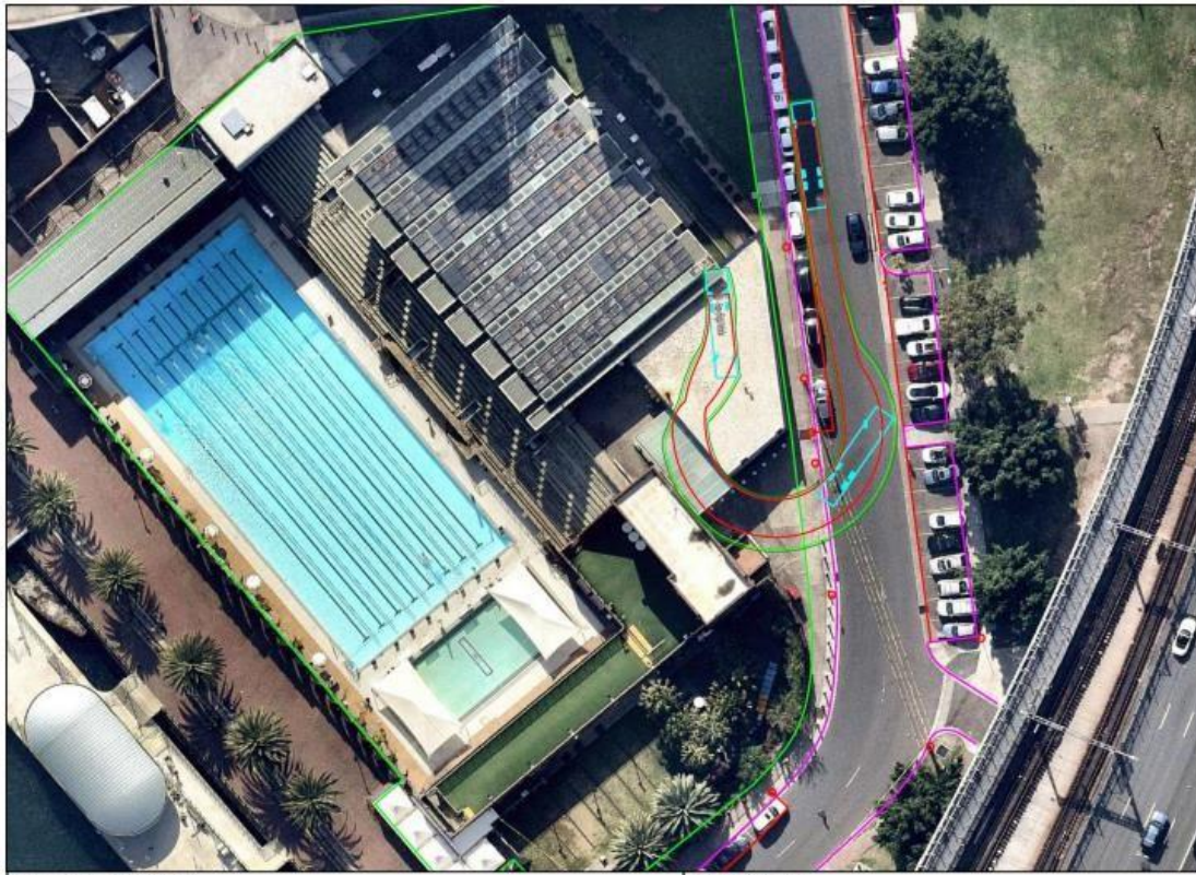
4 Alfred Street, Milsons Point Swept Path Diagram Site (Gate 2), Turn Left onto Alfred Street South 12.5 x 2.5m Heavy Rigid Vehicle (0.3m Clearance) Scale 1:500 @ A4 Plan Prepared by Jim's Traffic Control (Hornsby) Date 23/02/2021
