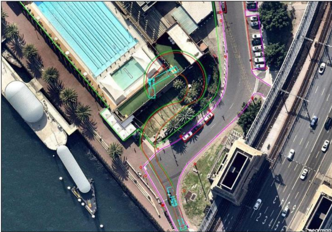
4 Alfred Street, Milsons Point Swept Path Diagram Olympic Drive, Turn Right into Site (Gate 1) 19 x 2.5m Articulated Vehicle (0.3m Clearance) Scale 1:500 @ A4 Plan Prepared by Jim's Traffic Control (Hornsby) Date 13/02/2021 Sheet 04
