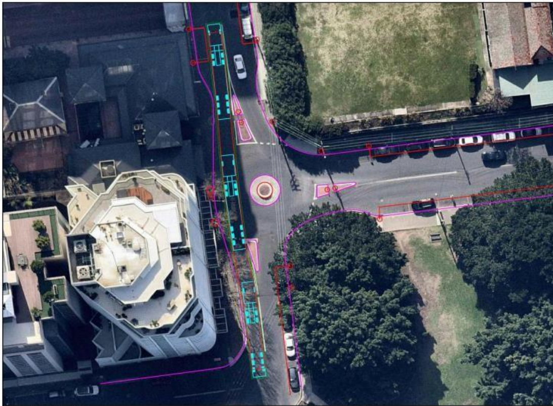
4 Alfred Street, Milsons Point Swept Path Diagram Alfred Street South, Continue onto Alfred Street South (Northbound) 19 x 2.5m Articulated Vehicle (0.3m Clearance) Scale 1:500 @ A4 Plan Prepared by Jim's Traffic Control (Hornsby) Date 13/02/2021
