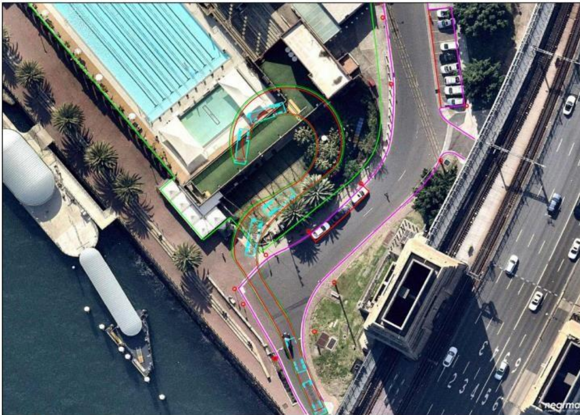
4 Alfred Street, Milsons Point Swept Path Diagram Olympic Drive, Turn Right into Site (Gate 1)
