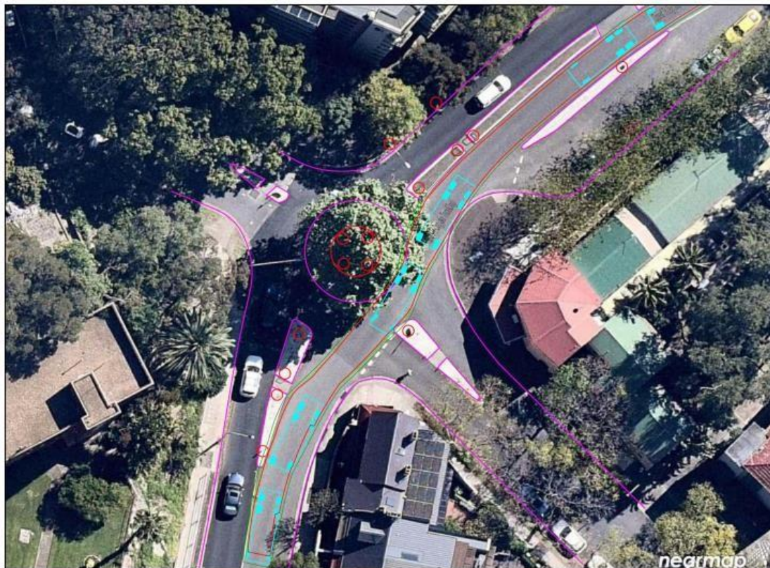
4 Alfred Street, Milsons Point Swept Path Diagram Clark Road, Continue onto Broughton Street 19m x 2.5m Truck and Dog (Trailer Combination) Centre Articulation (0.3m Clearance) Scale 1:500 @ A4 Plan Prepared by Jim's Traffic Control (Hornsby) Date 23/02/2021
