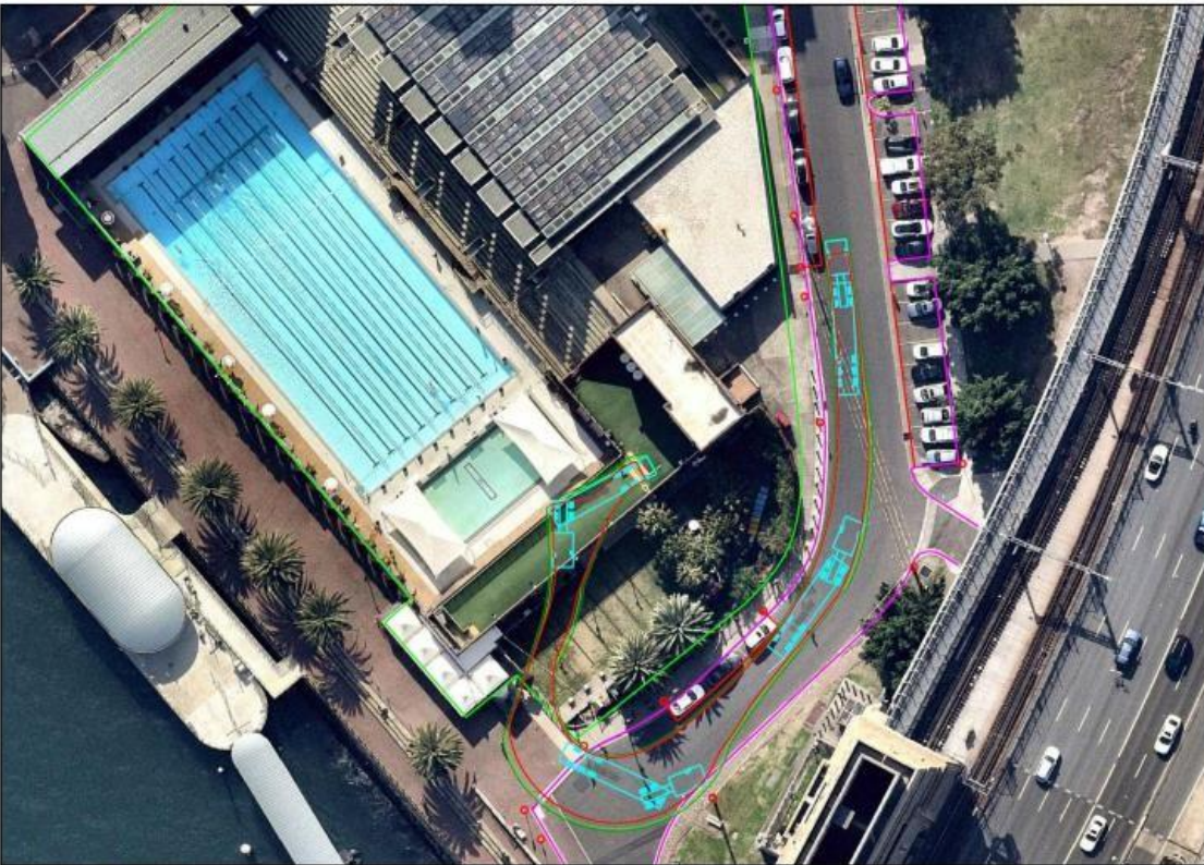
4 Alfred Street, Milsons Point Swept Path Diagram Site (Gate 1), Turn Left onto Alfred Street South 19 x 2.5m Articulated Vehicle (0.3m Clearance) Scale 1:500 @ A4 Plan Prepared by Jim's Traffic Control (Hornsby) Date 13/02/2021 Sheet 05
