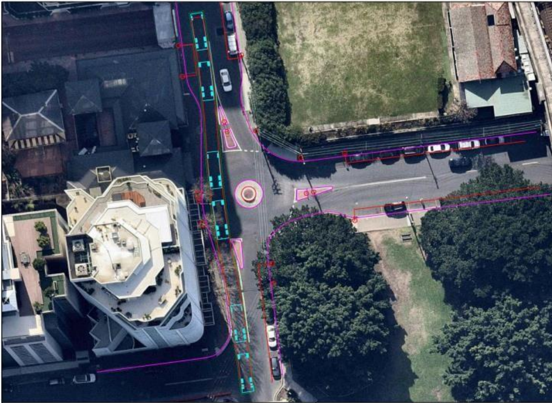
4 Alfred Street, Milsons Point Swept Path Diagram Alfred Street South, Continue onto Alfred Street South (Northbound) 19m x 2.5m Truck and Dog (Trailer Combination) Centre Articulation (0.3m Clearance) Scale 1:500 @ A4 Plan Prepared by Jim's Traffic Control (Hornsby) Date 23/02/2021
