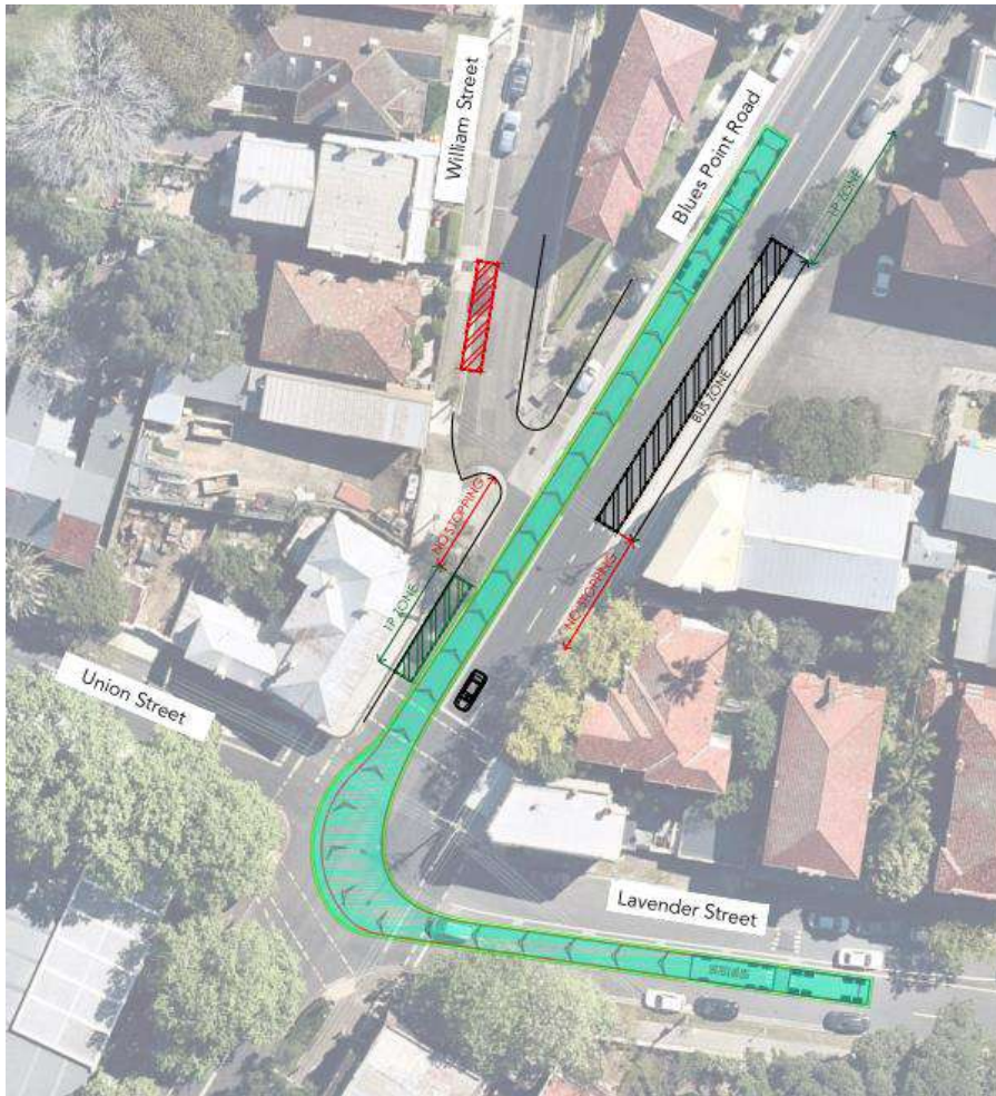
Figure 32 - Truck and Dog Swept Path in the Event that the Southbound Lane is Occupied
