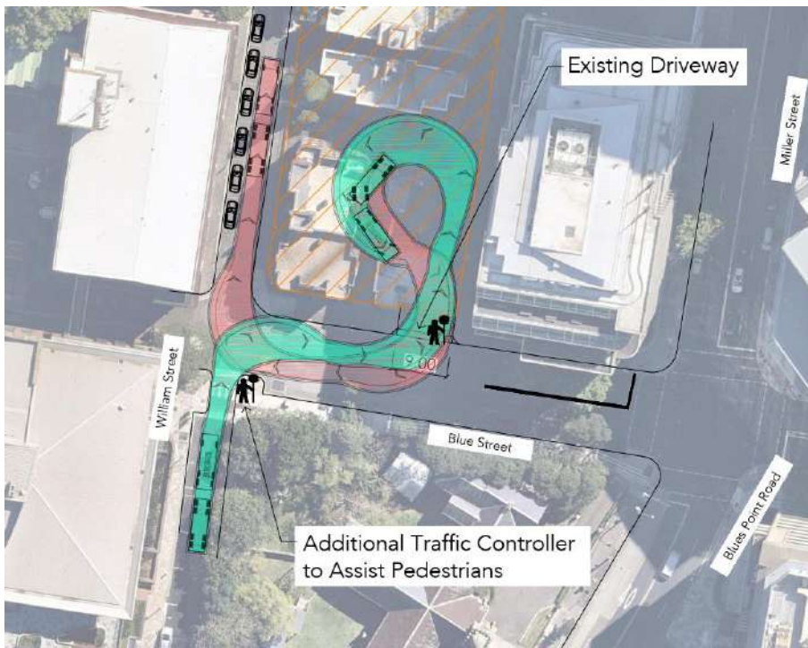
Figure 26 - Truck and Dog Access and Egress into and out of the Site (Assisted by an Accredited Traffic Controller)
