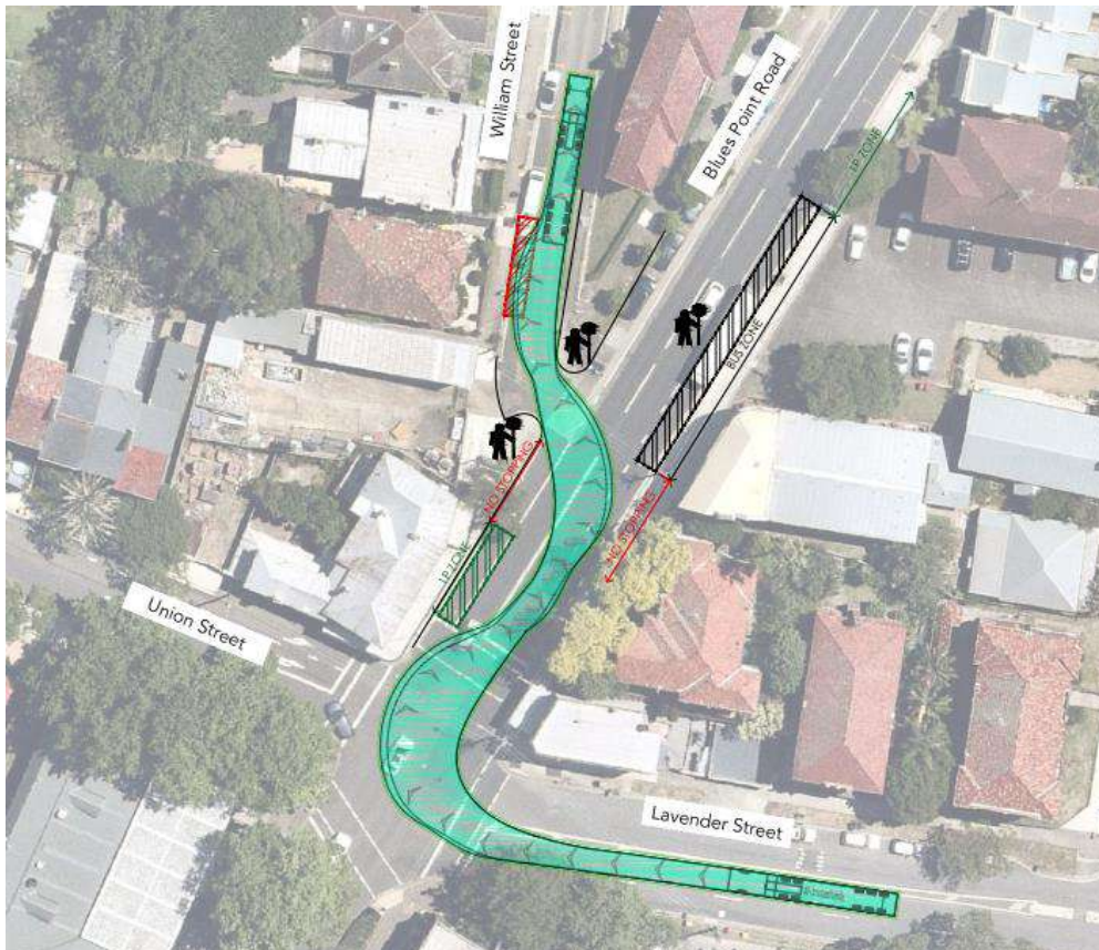
Figure 29 - 19m AV (Sem-Trailer) Turning Right from Lavender Street into Blues Point Road then Left into William Street (Managed by Accredited Traffic Controllers)
