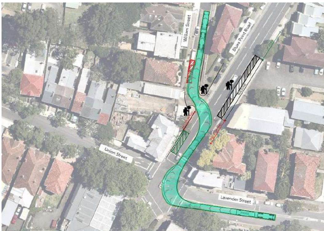
Figure 25 - Truck and Dog Turning Right from Lavender Street into Blues Point Road then Left into William Street (Managed by Accredited Traffic Controllers)
