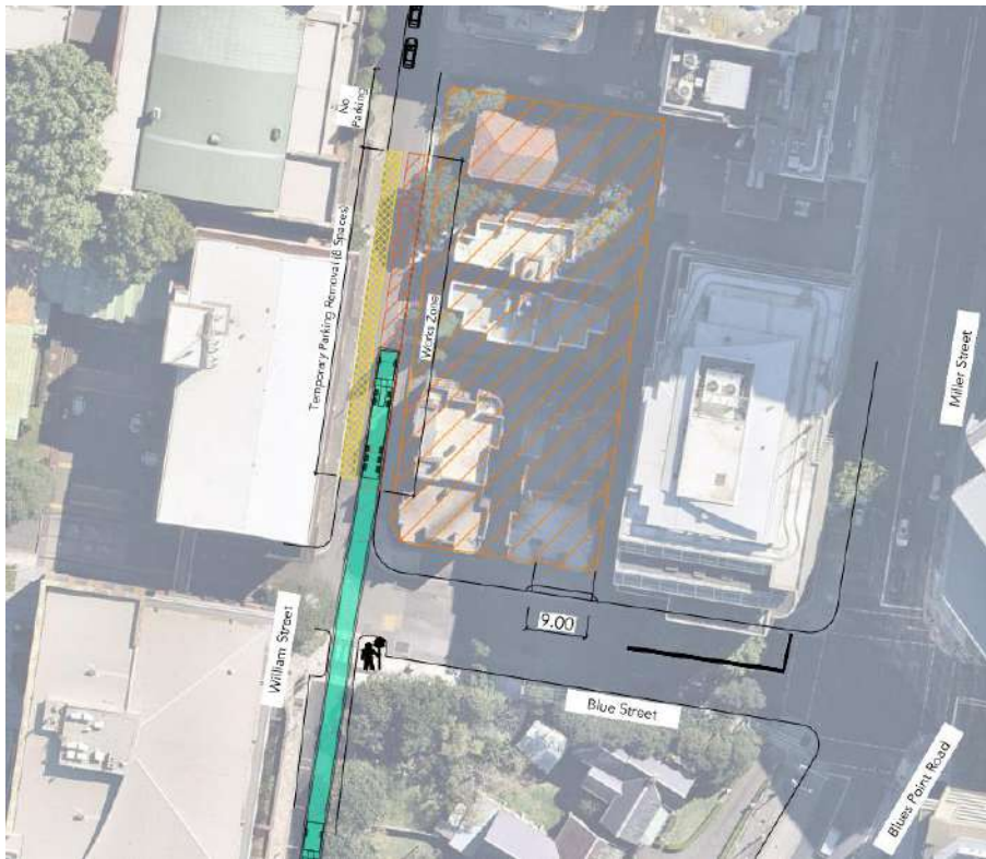
Figure 30 - AV (Sem-Trailer) Access into the Works Zone on William Street
