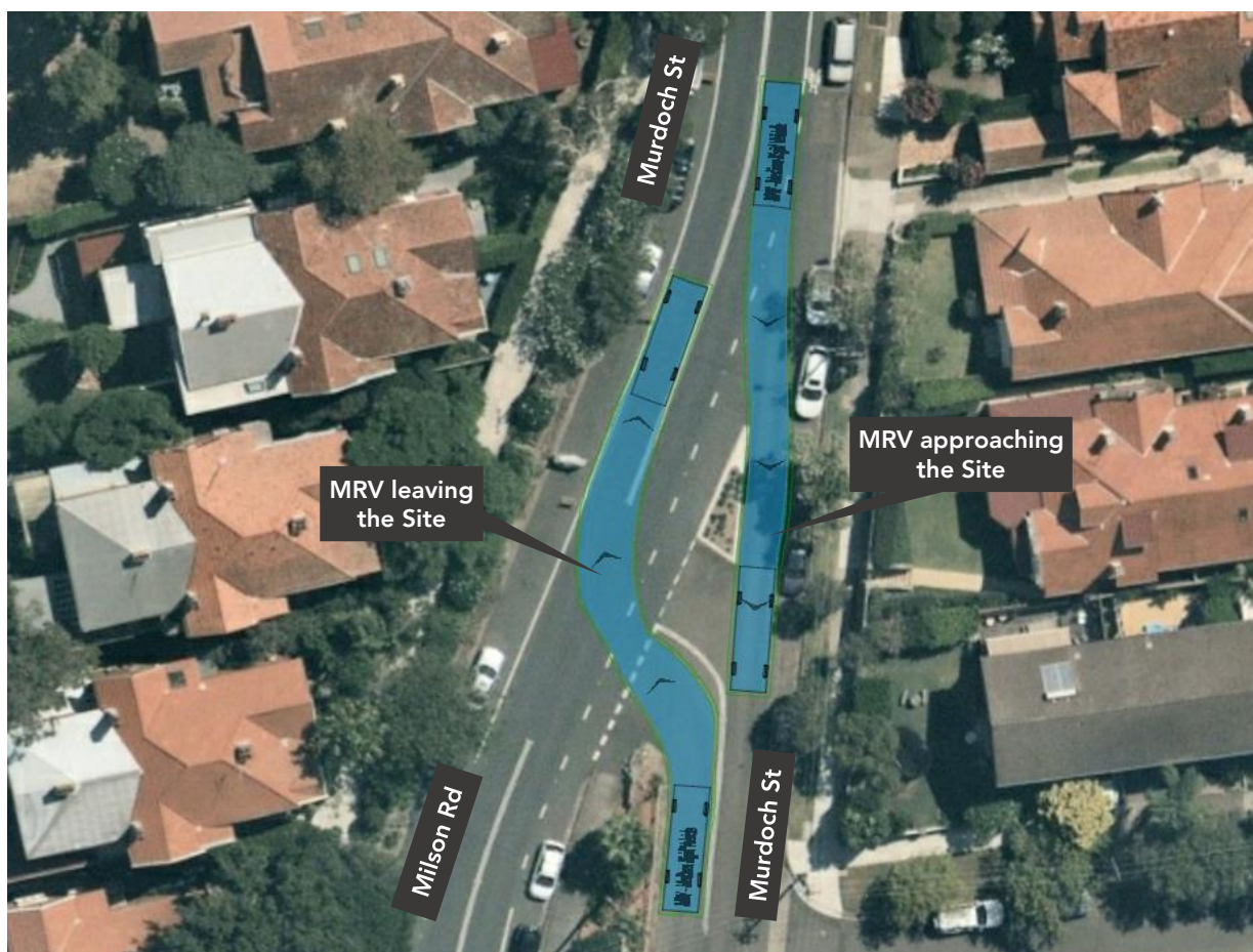
Figure 16 – MRV at Murdoch St / Milson Rd Intersection
