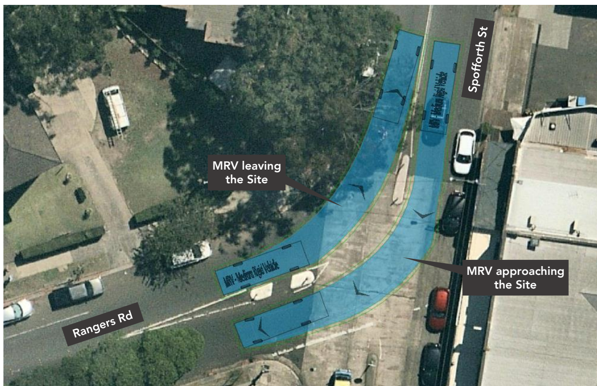
Figure 19 – MRV at Rangers Rd / Spofforth St Intersection
