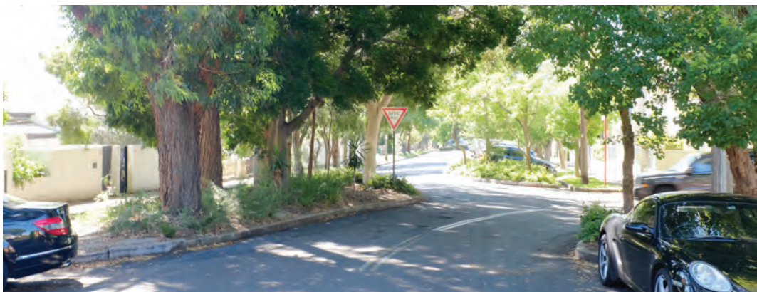
Hayberry street traffic calming incorporates kerb blisters planted with large canopy trees to create a distinctive streetscape that effectively restricts traffic speeds
