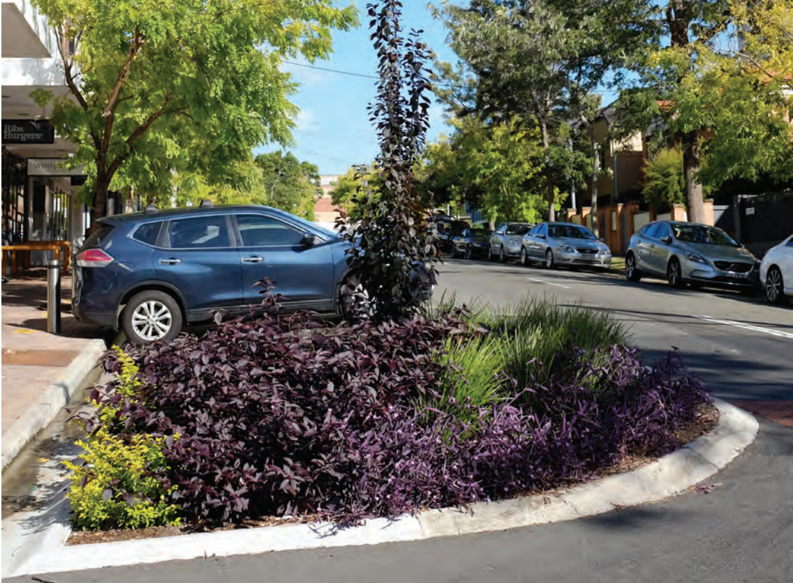
Well designed traffic control measures such as kerb blisters provide opportunities for tree planting to help combat the urban heat island effect of surrounding hard surfaces.
