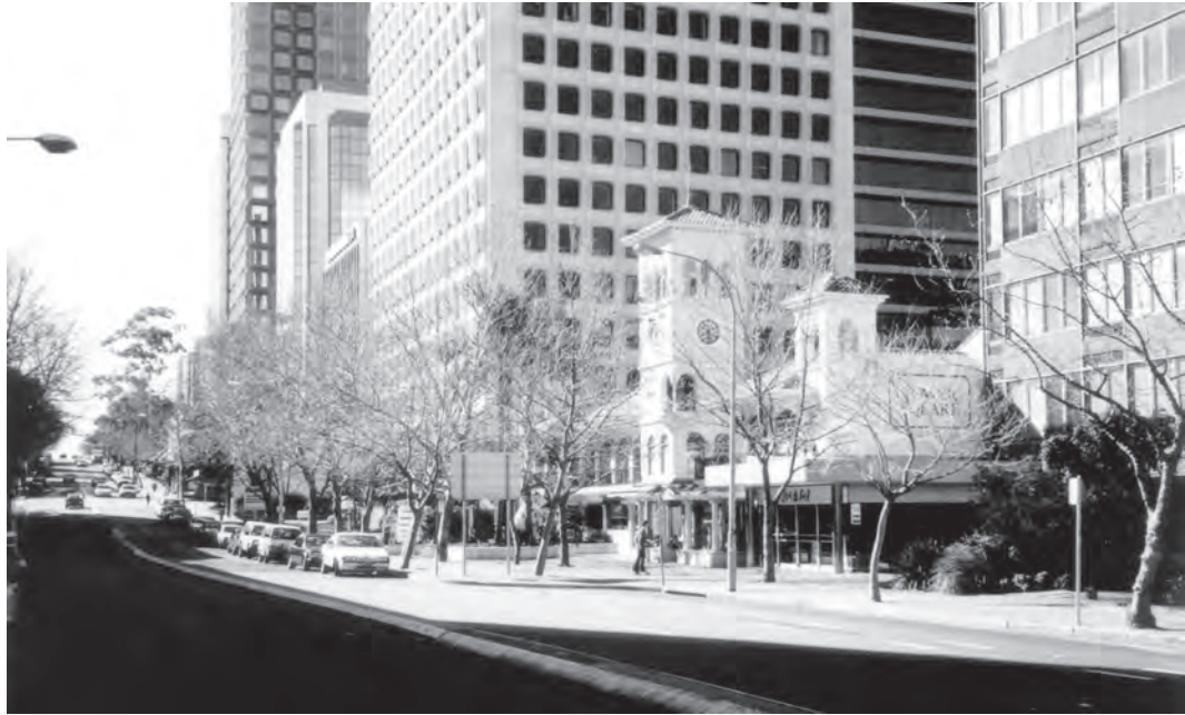
Deciduous Plane trees in Miller St allow sunlight into the North Sydney CBD during the cooler winter months.
