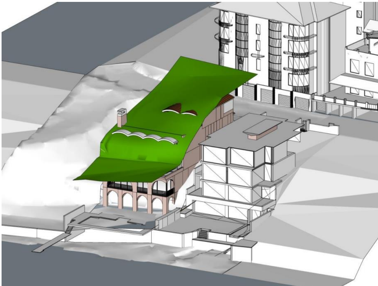
Figure 1. Extract from written request of the proposed protrusions through the height plane
