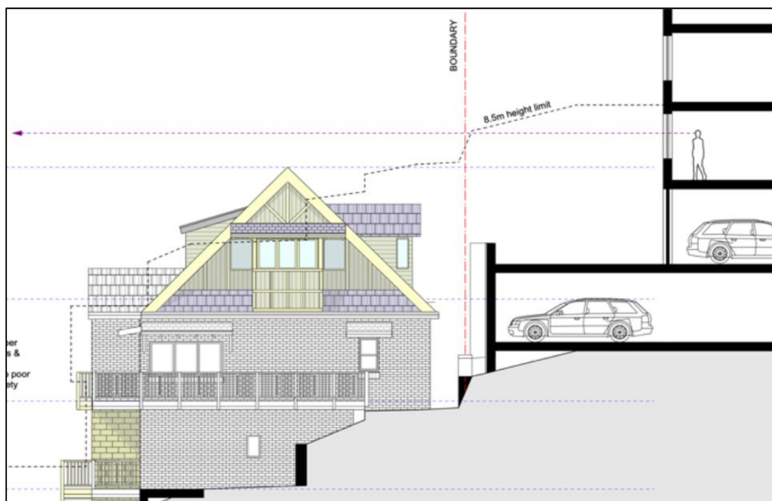
Figure 16: Western elevation plan of the proposal showing the level difference between the subject site and No. 74-78 Cairo Street to the south (left).
