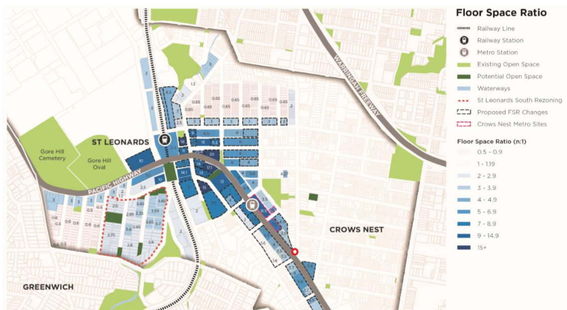
Figure 13 – Extract from the 2036 Plan in respect of indicative changes to floor space ratio. The red circle indicates the location of the subject site.
