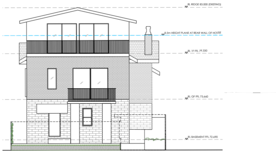
Figure 2 Existing rear elevation - blue line indicating NS LEP 2013 Height Control Source: Noble Architecture
