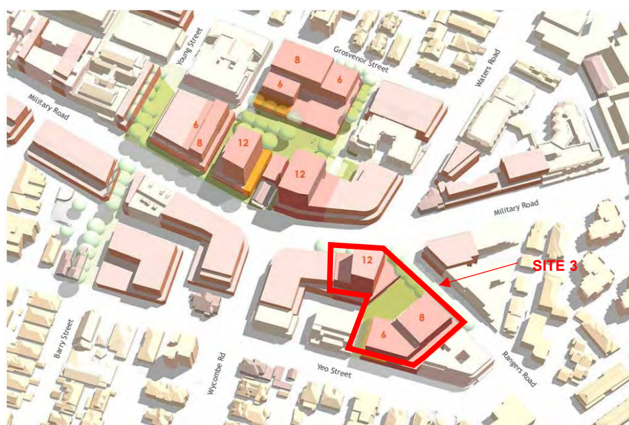
FIGURE 2: Recommended building envelope for 'opportunity sites' in Neutral Bay Town Centre (source: Rescinded MRCPS, p. 52)
