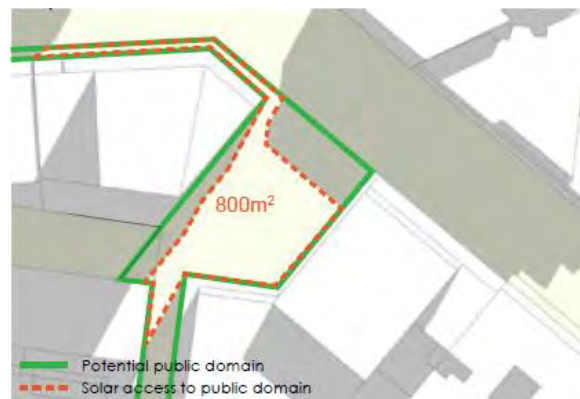
FIGURE 39: Solar impact on Rangers Road Plaza under rescinded MRCPS controls. (10am, 21 June).
