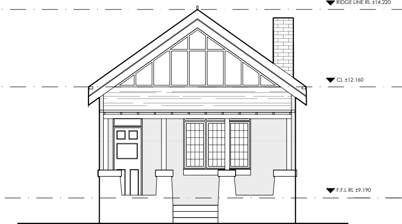
4 ELEVATION - EXISTING NORTH SCALE 1:100
