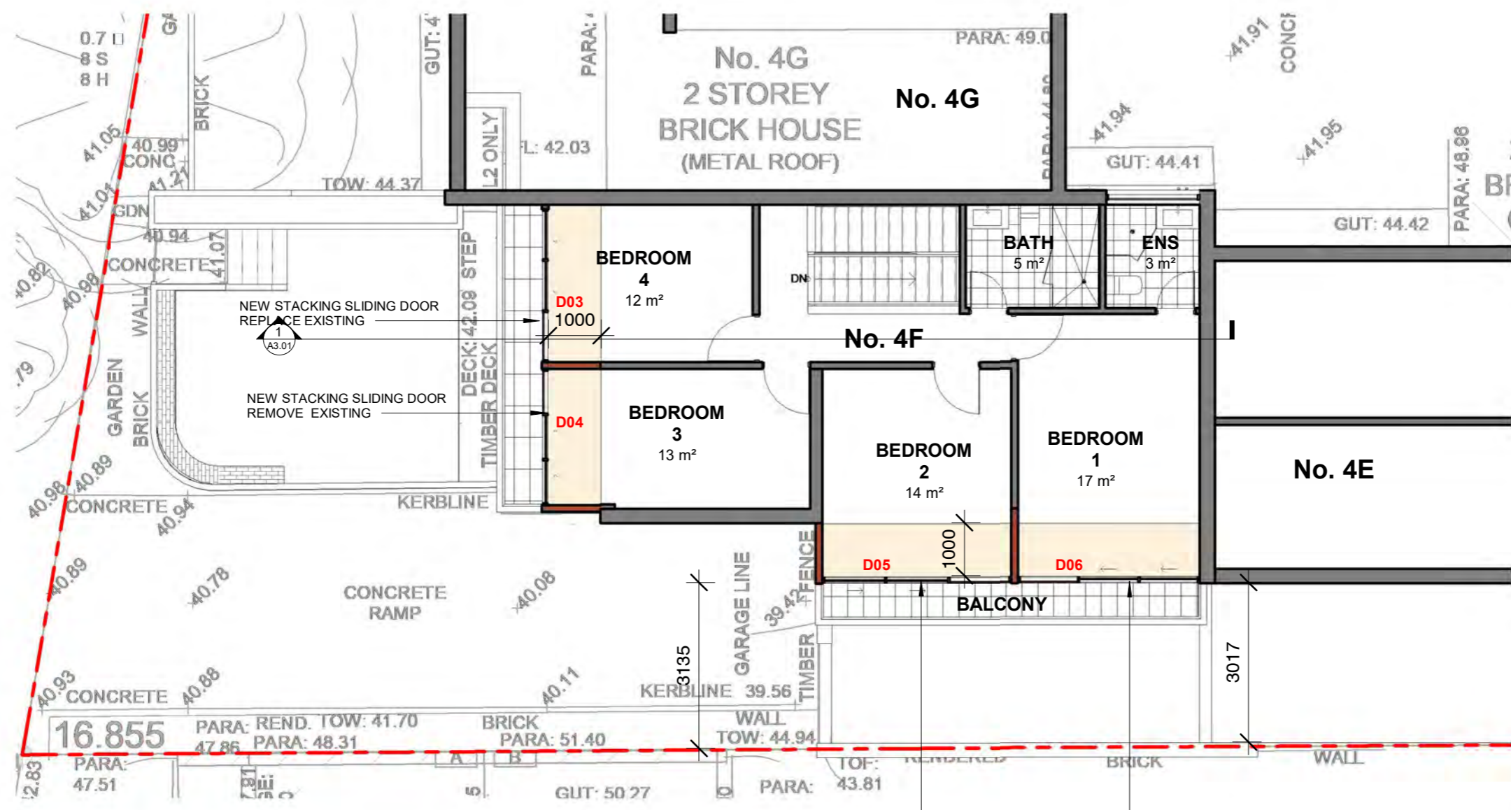
1 LEVEL 1 FLOOR PLAN A2.01 1 : 100
