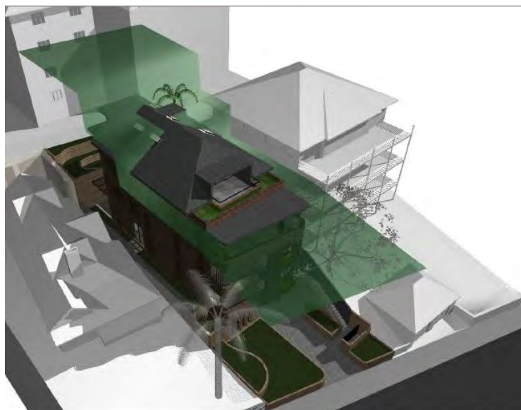
Figure 37. Height Plane Diagram indicating the extent of the existing and proposed variations
