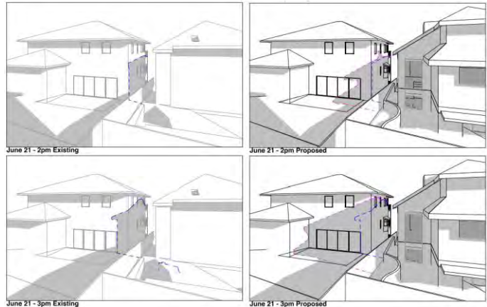
Figure 52. Additional overshadowing to north eastern rear elevation and courtyard of No. 7 Undercliff Street at 2:00pm & 3:00pm in midwinter.
