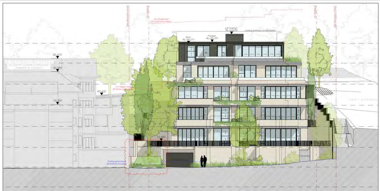
Figure 13: North Elevation, detailing deep soil zone which will accommodate mature tree planting to provide acoustic and visual privacy to 8 Sutherland Street (Source: MHN Design Union)
