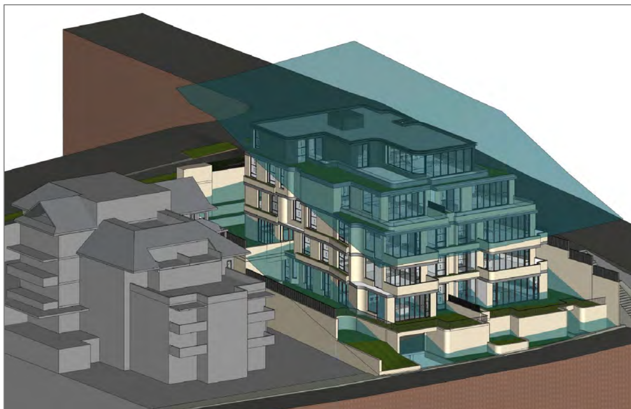
Figure 3: Height Plane Diagram based on 12m extrapolated height limit (Source: MHN Design Union)
