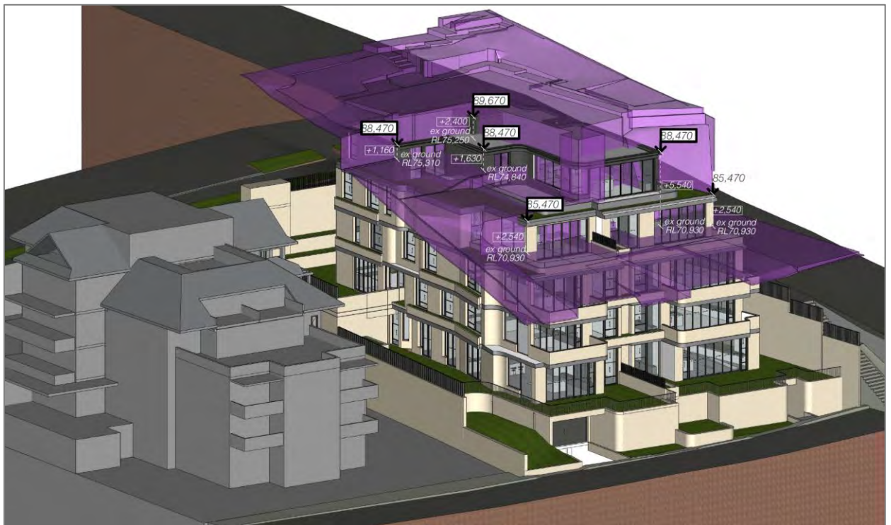
Figure 4: Height Plane Diagram based on height measured from ground level (existing). The purple plane denotes the 12m height standard (Source: MHNDU)
