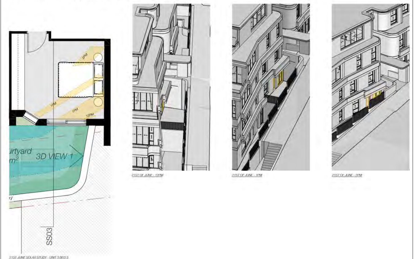
Figure 11: Extract of DWG No. 9413 – demonstrating proposed amendments to provide improved solar access into Unit 3 Bedroom 4 (Source: MHNDU)
