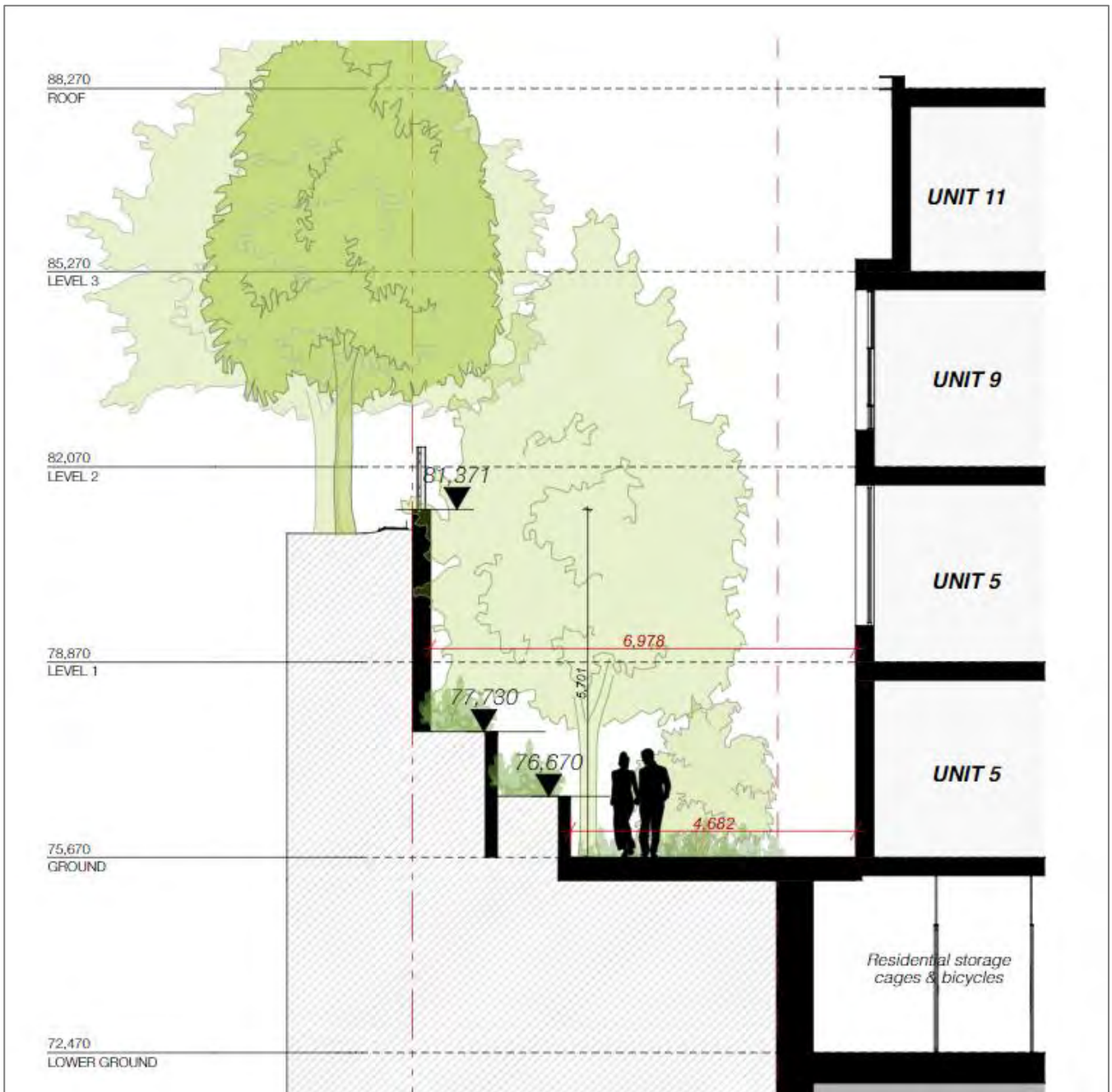
Figure 18: Extract of DWG 9417 which demonstrates that the east facing bedrooms are located 6.978m from the wall on the eastern boundary. The east facing bedrooms are located at a level of RL 78.87 and the wall on the eastern boundary is at a level of RL 83. 371. The living room is located 4.682m from the wall which provides sufficient room for ventilation and privacy (Source: MHNDU)
