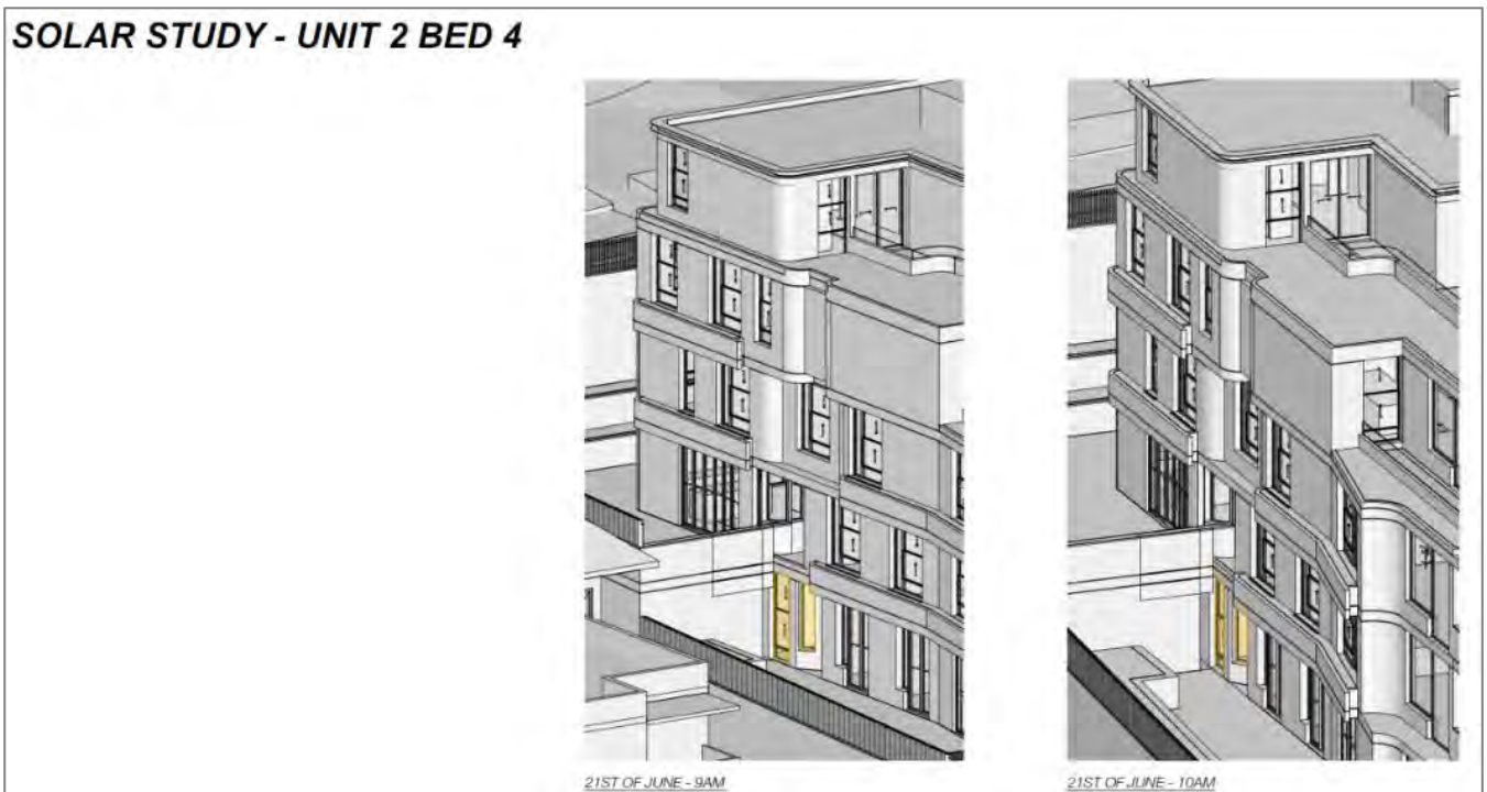
Figure 6: Extract of DWG No. 9407 – demonstrating proposed amendments to provide improved solar access into Unit 2 Bedroom 4 (Source: MHNDU)
