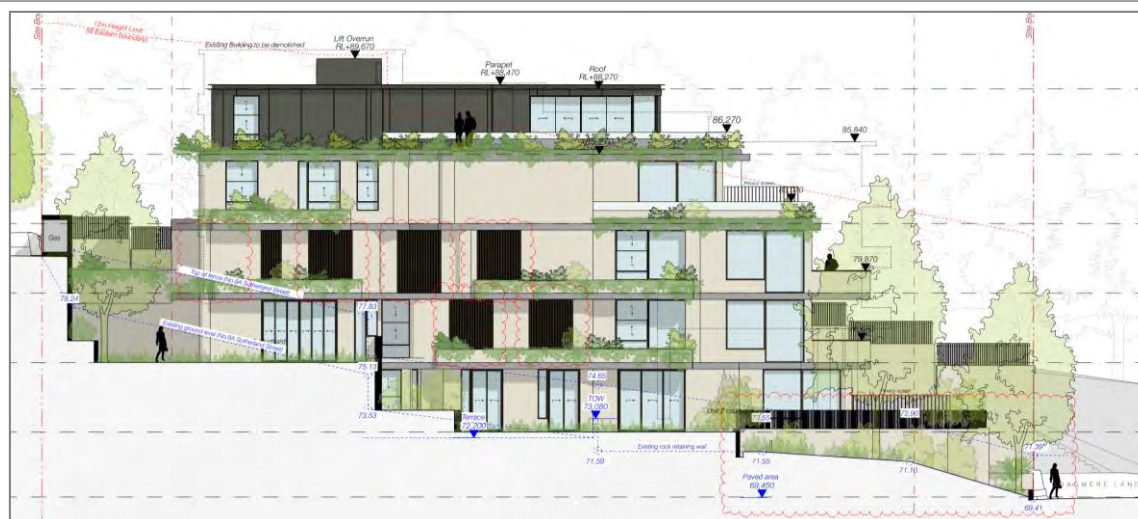
Figure 18: East Elevation, showing proposed 2-3 storey built form to Grasmere Lane, and 3 storey built form to Sutherland Street (Source: MHNDU)
