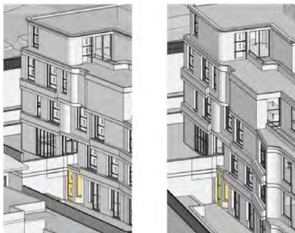
Figure 54. Solar access to rear bedroom of unit 2 at 9:00am and 10:00am in mid-winter
