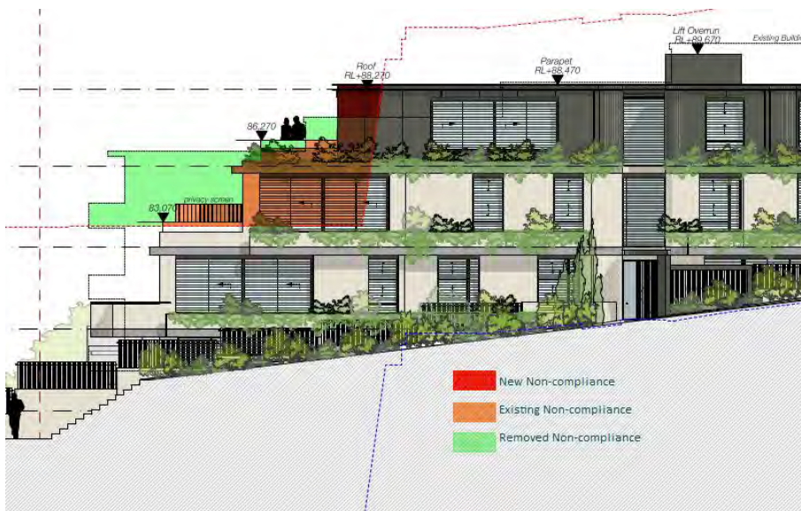
Figure 45. Comparison of proposed and existing non-compliances as illustrated on the western (Park Avenue) elevation
