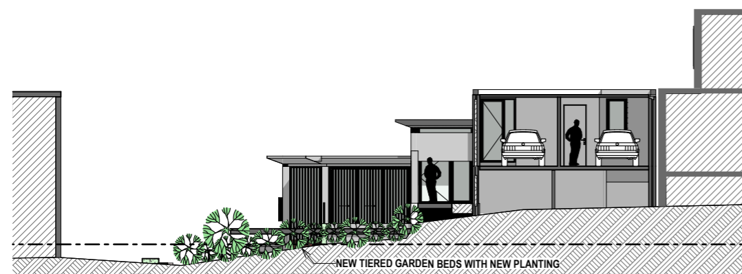
EAST ELEVATION & SECTION THROUGH GARAGES
