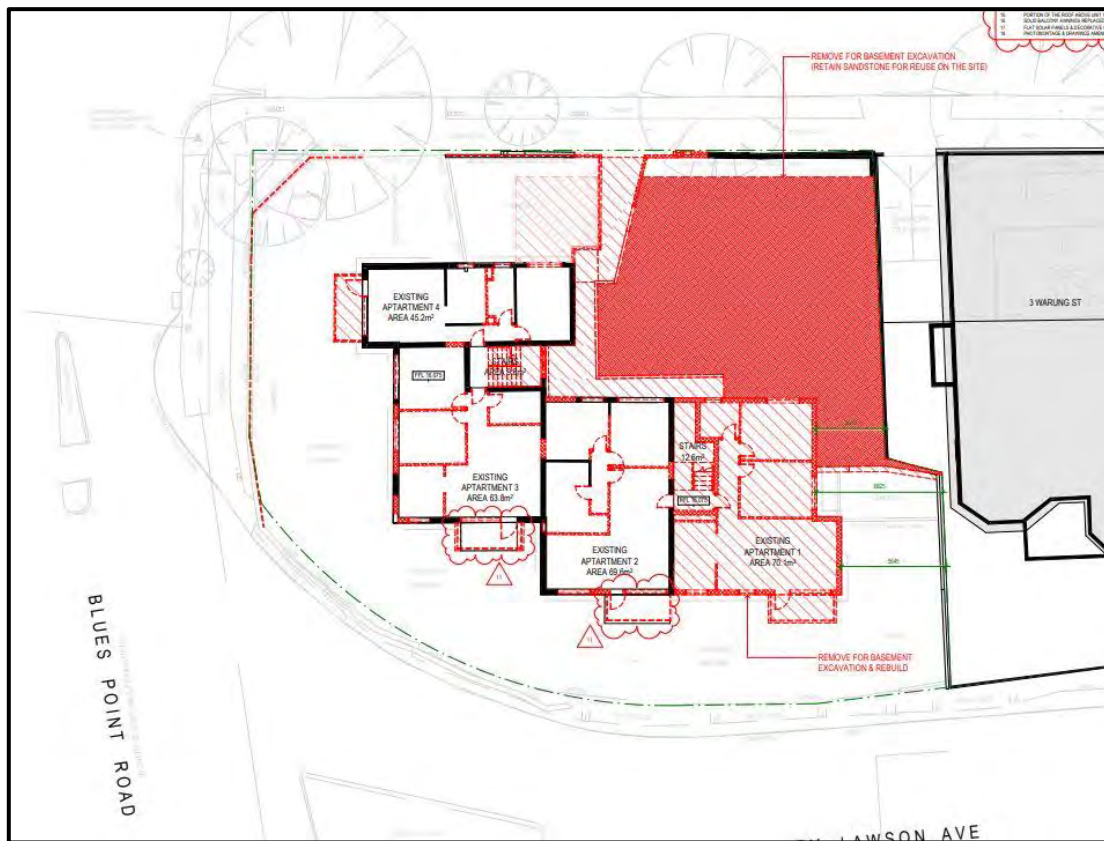
Figure 3: Demolition plan – existing ground floor
