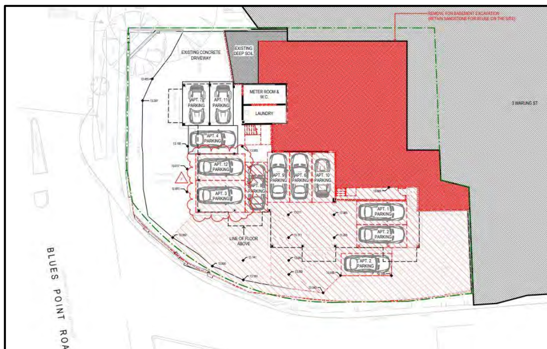
Figure 2: Demolition plan – existing lower ground floor
