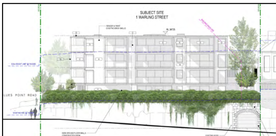
Figure 3: Extract of south elevation (Warung St frontage) showing LEP 8.5m height line (Source: Squillace Architecture, Project No. HIG2009)
