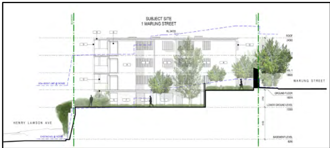
Figure 4: Extract of east elevation (from No. 3 Warung St) showing LEP 8.5m height line (Source: Squillace Architecture, Project No. HIG2009)
