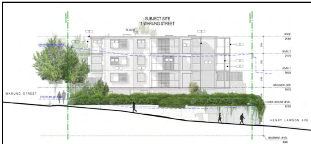
Figure 5: Extract of west elevation (Blues Point Road) showing LEP 8.5m height line (Source: Squillace Architecture, Project No. HIG2009)
