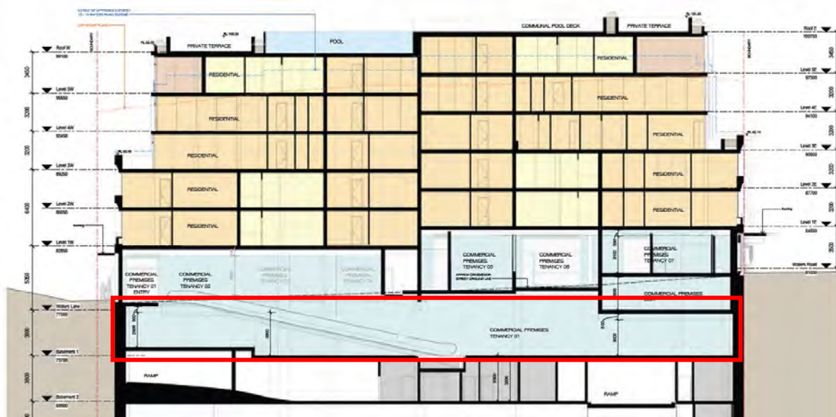
FIGURE 10: Section plan of concept design with underground commercial area outlined in red (Source: SJB 2021 with additions by Council Officer).
