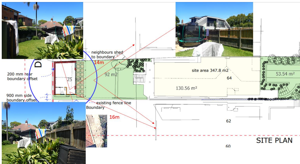
Figure 21 – Annotated Site Plan with photos considering the existing/proposed views and privacy between adjoining properties.
