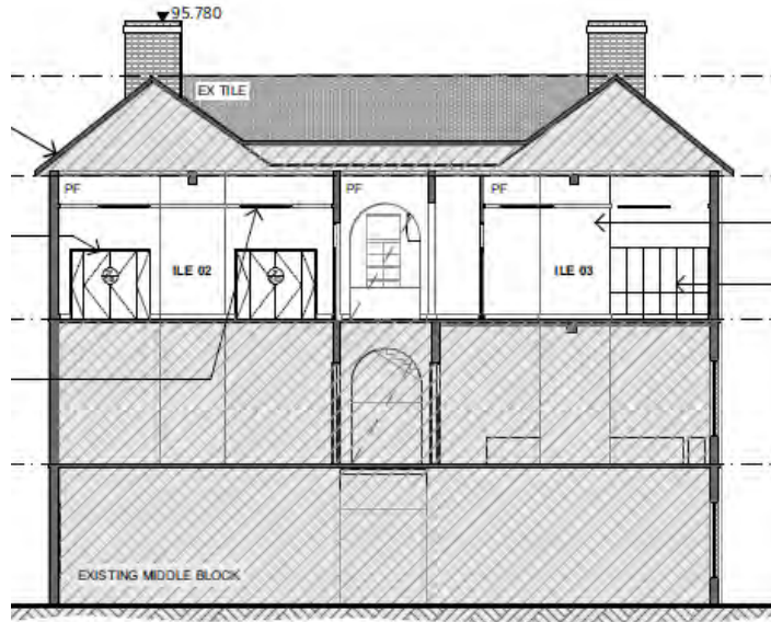
Figure 32: Proposed north-south section Elevation. (Source: SHAC Architects)
