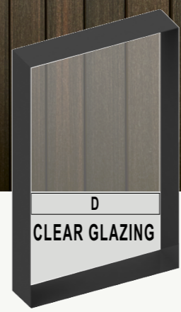
E WINDOW SHROUD DULUX BLACK SATIN 9109024S POWDER COATING OR SIMILAR WINDOWS ON THE EAST AND WEST FACADE
