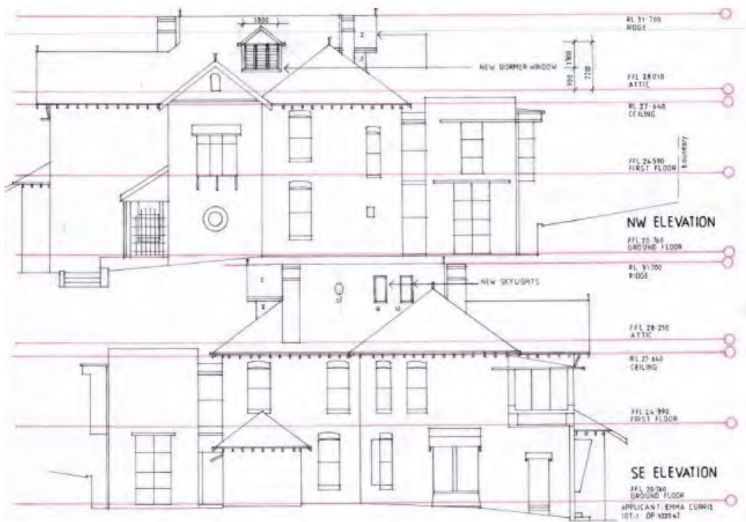
Figure 4. Proposed North Western and South Eastern Elevations
