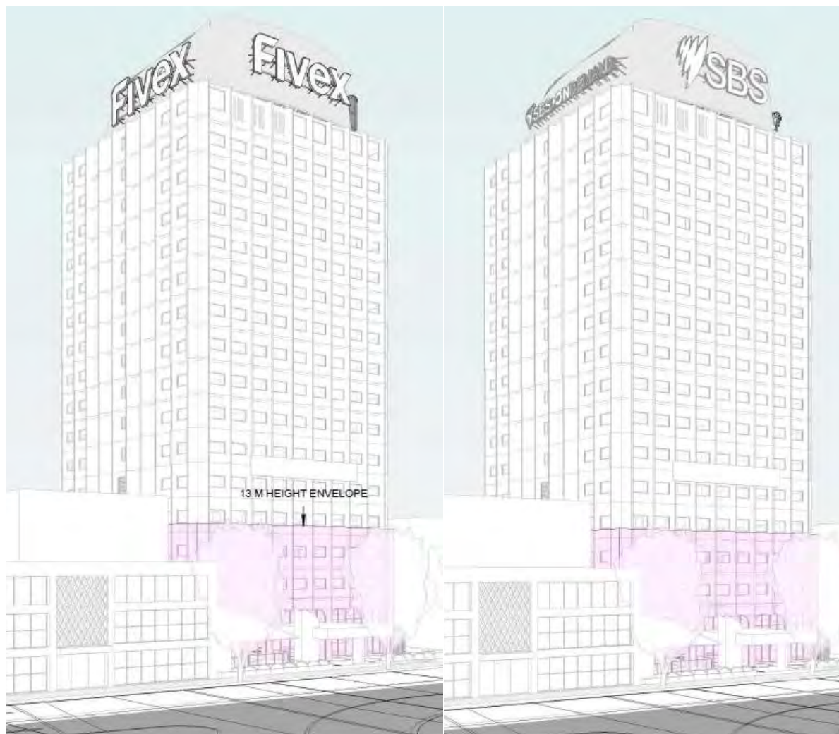
Figure 1 Existing and proposed comparison (maximum height 60.75m) with 13m height line shown.
