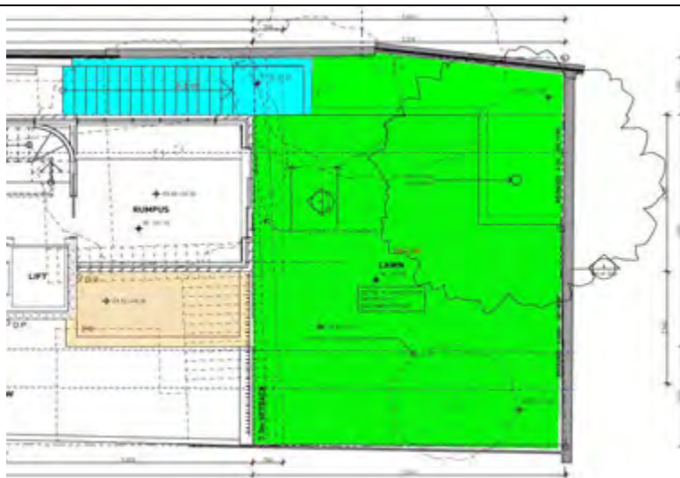
Compliance diagrams – landscaped area (shaded in green) and un-built upon area (shaded in cyan)
