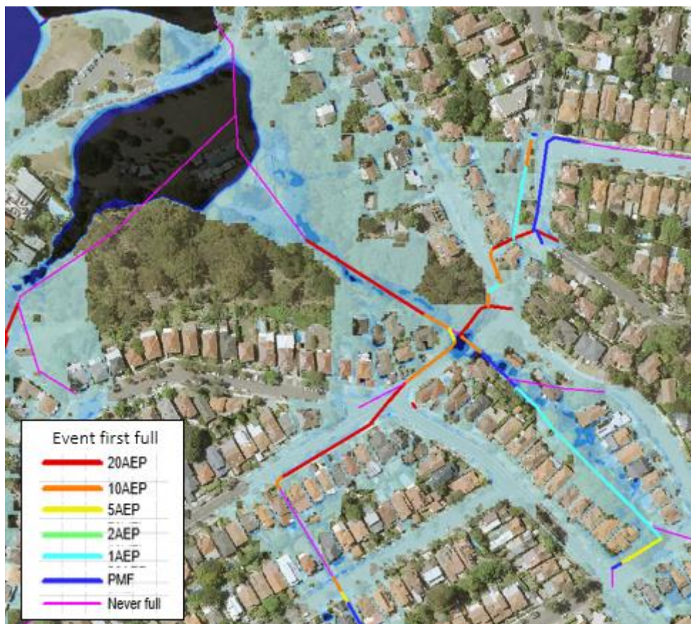
Image 39: Reynolds Street Drainage Capacity
