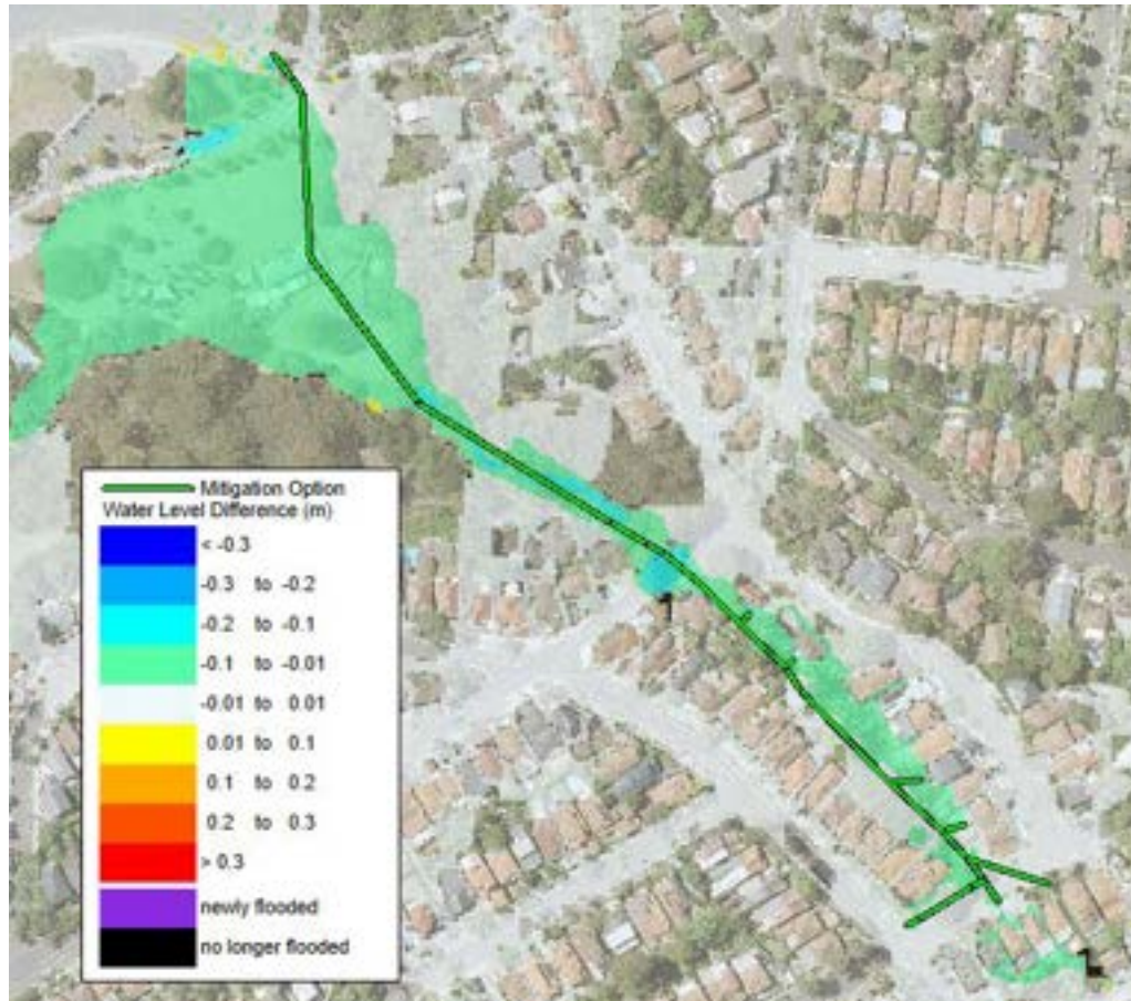
Image 40: Reynolds Street Drainage Upgrade (FM-N06) – 1% AEP Impact
