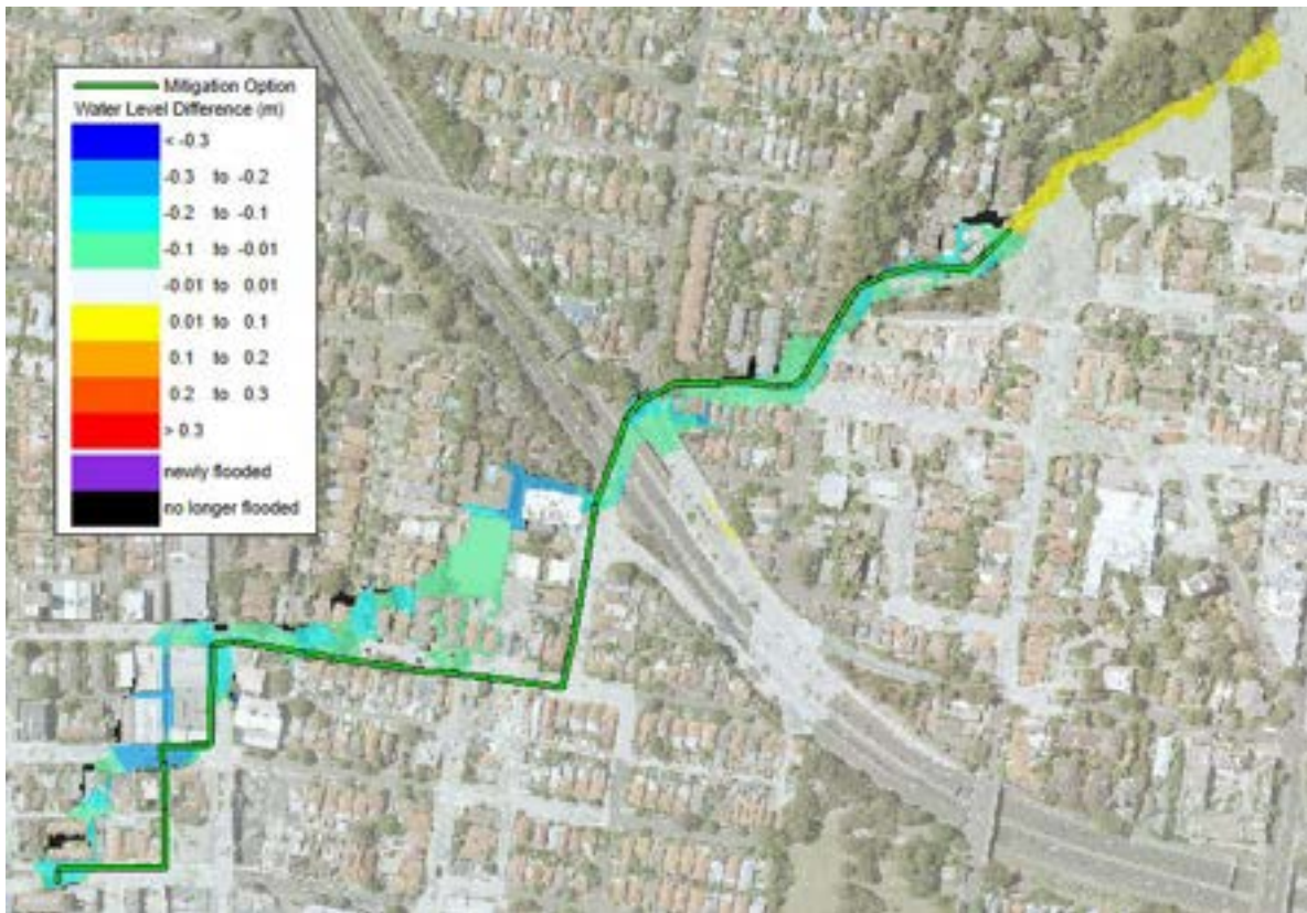
Image 34: Trunk Upgrade from Albany Street to Flat Rock Creek (FM-N01) – 1% AEP Impact
