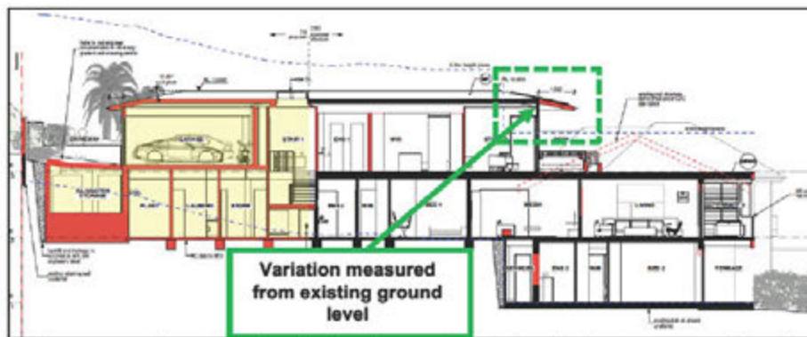
Figure 3: Long section drawing indicating extent of variation to upper-level roof form above rooftop deck
