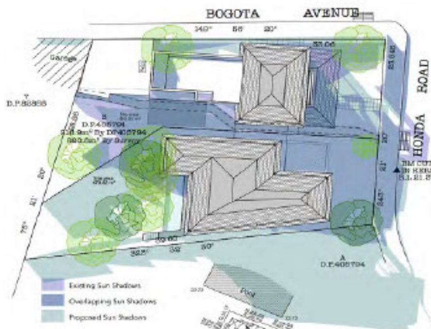
Figure 14 - Shadow Diagram at 9.00am in mid-winter (June 21) detailing shadow cast from the Dwelling 1 (subject to alterations and additions) and Dwelling 2 (new dwelling) – DA27 Rev B
