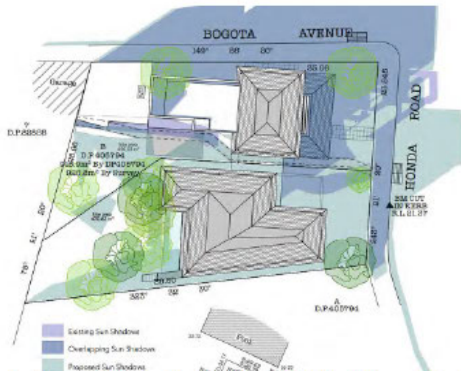
Figure 17 - Shadow Diagram at 3pm in mid-winter (June 21) detailing shadow cast from the Dwelling 1 (subject to alterations and additions) and Dwelling 2 (new dwelling) – DA30 Rev B
