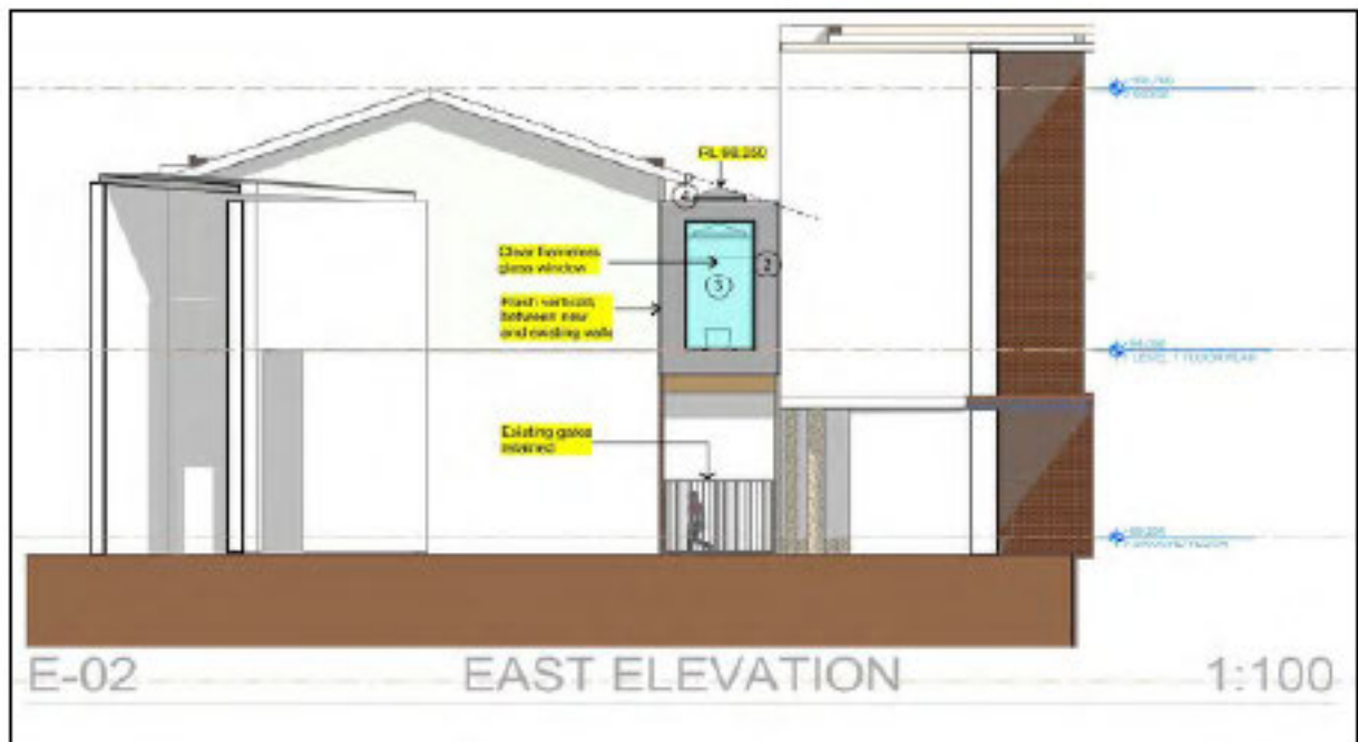
Figure 6: East (rear) elevation
