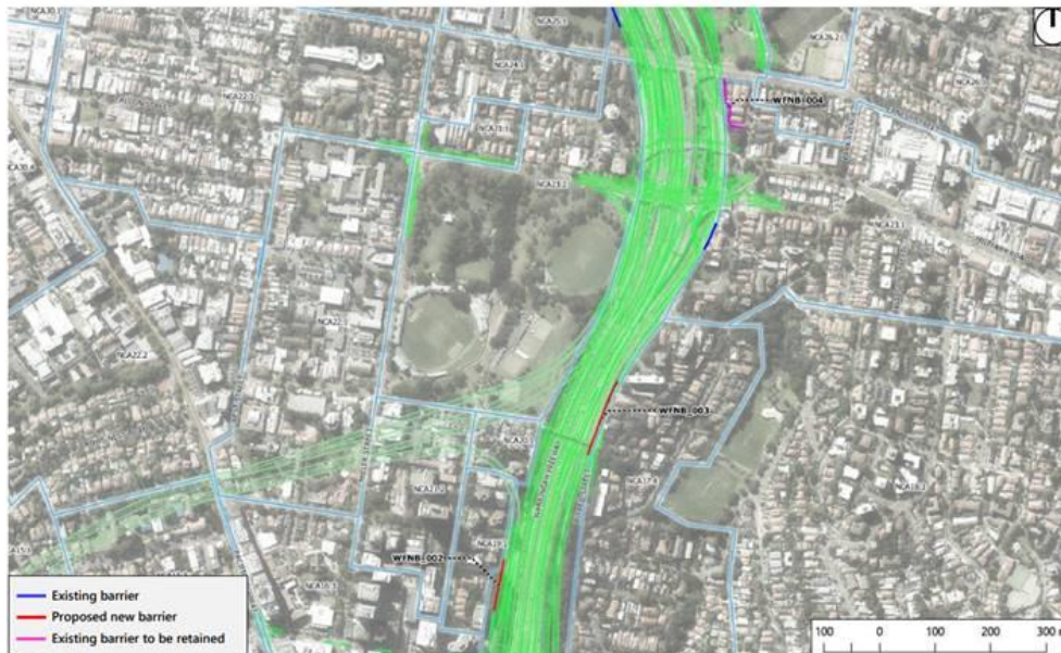
Figure 7-2 – Noise barriers considered in the NMG analysis at Warringah Freeway and surrounds (centre)
