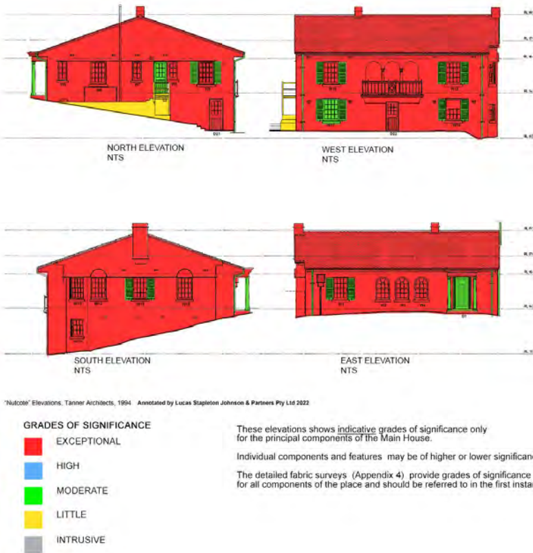
Figure 5. 2: Elevation plans showing indicative grades of significance for the principal components of the Main House of Nutcote.
