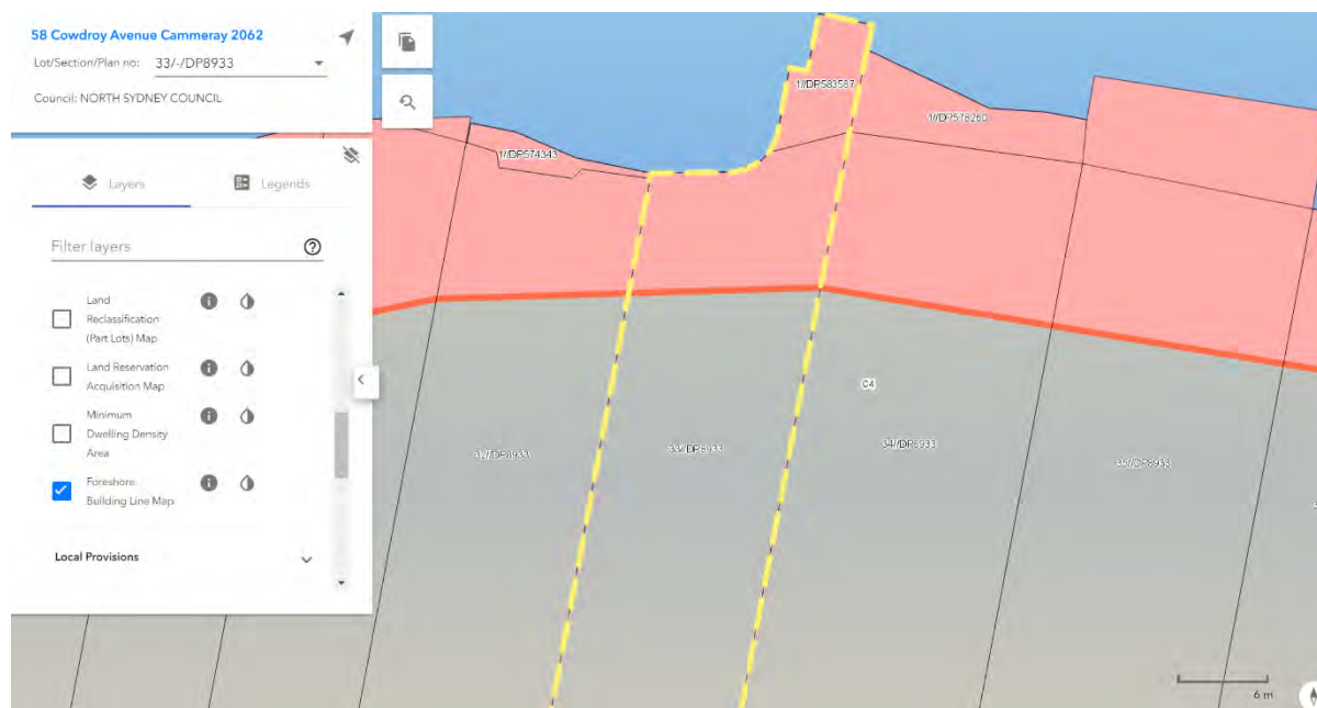
Figure 57: Map of foreshore building line (red) and the foreshore area (shaded red) as it applies to the site (outlined dashed yellow) (Source: NSW Spatial Viewer)
