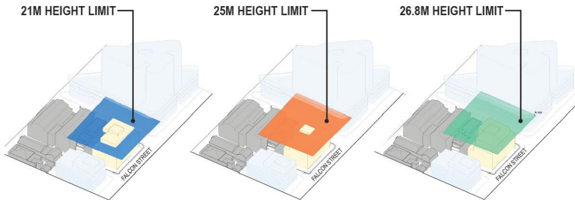
Figure 14: Building Height Plane of indicative concept accompanying the Planning Proposal. (Drew Dickson Architects, September 2022).
