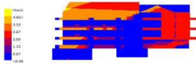
East elevation - Daylight hours received by 45 McLaren Street with 168 Walker Street DA scheme only.
