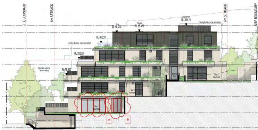
Figure 4. Proposed Western Elevation (at the building line behind existing footpath retaining wall)
