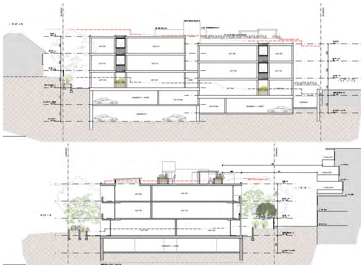
Sections through the proposed building showing the roof terrace, three residential levels and the basement. In the lower drawing, to the right is part of the 3 – 5 storey flat building at 130 Spencer Road, north of the site.
