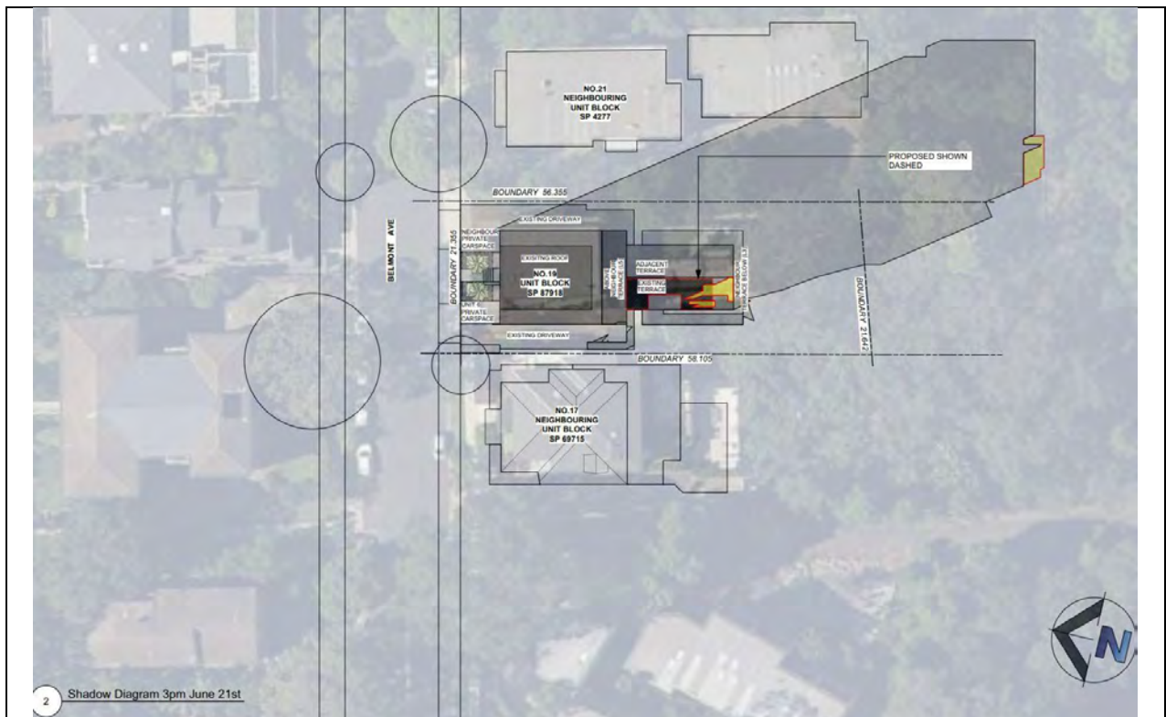
Shadow diagrams – at 9am (top), 12pm (centre) and 3pm (bottom) during mid-winter (21 June)
