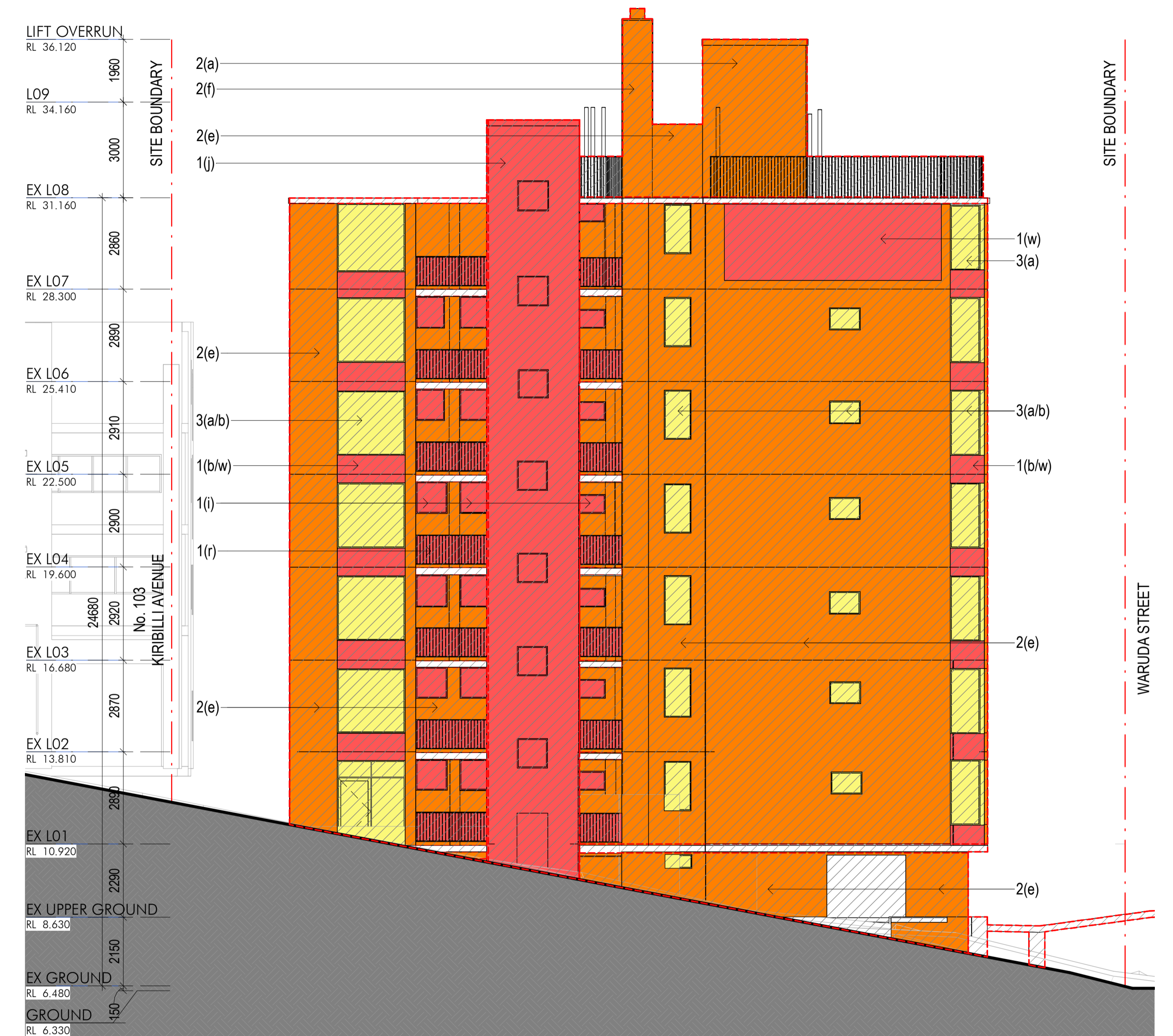
2 DEMOLITION - ELEVATION - WEST 1:100 96.6% OF FACADE EFFECTED BY NON-COMPLIANCE
