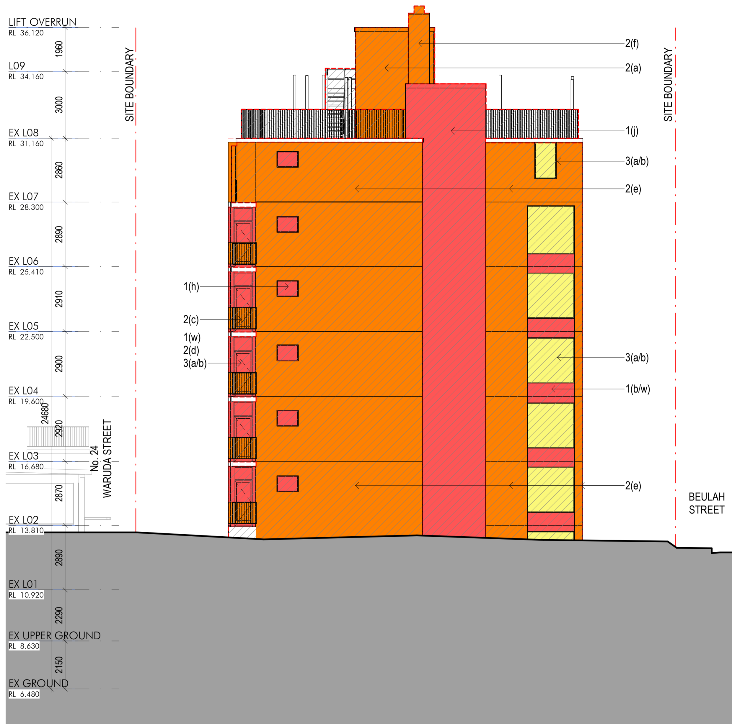
1 DEMOLITION - ELEVATION - NORTH 1:100 98.75% OF FACADE EFFECTED BY NON-COMPLIANCE
