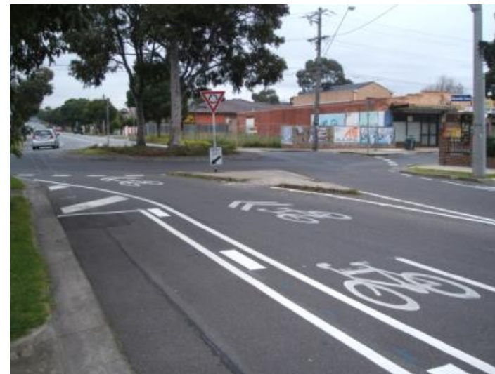
Figure 6.12: Possible Trial for Alternate Roundabout Markings
