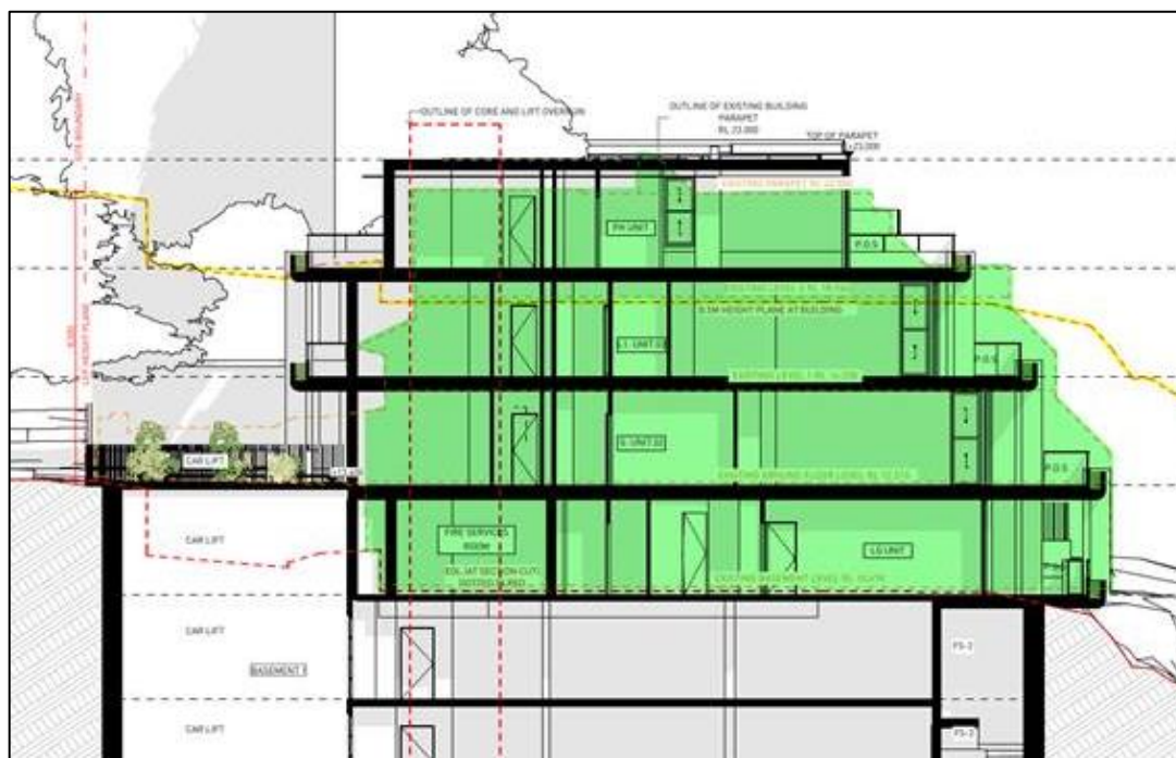
Figure 28a: Existing and proposed building shown shaded with 8.5m height standard depicted in yellow.
