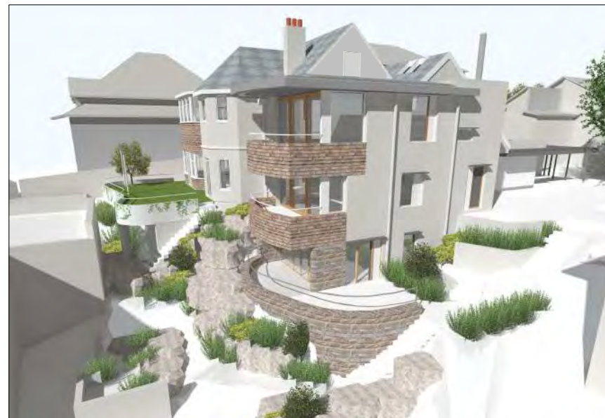
4 3D View - North Elevation BALUSTRADES TO NEW BALCONIES CHANGED FROM FLAT FACED TO BOW - FRONTED
