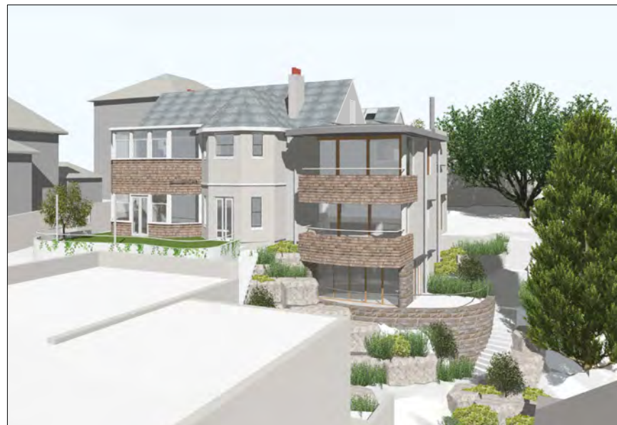
2 3D View - North East Elevation BALUSTRADES TO NEW BALCONIES CHANGED FROM FLAT FACED TO BOW - FRONTED
