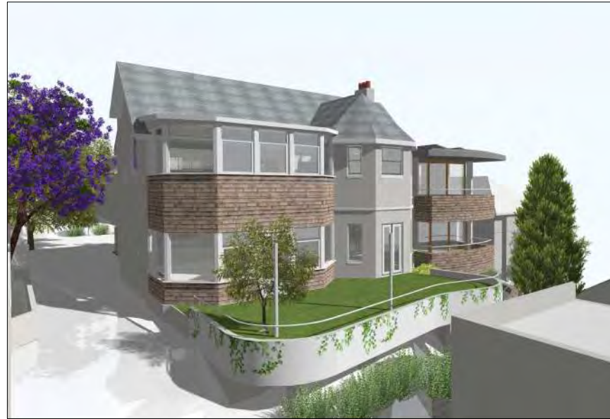
1 3D View - South East Elevation BALUSTRADES TO NEW BALCONIES CHANGED FROM FLAT FACED TO BOW - FRONTED
