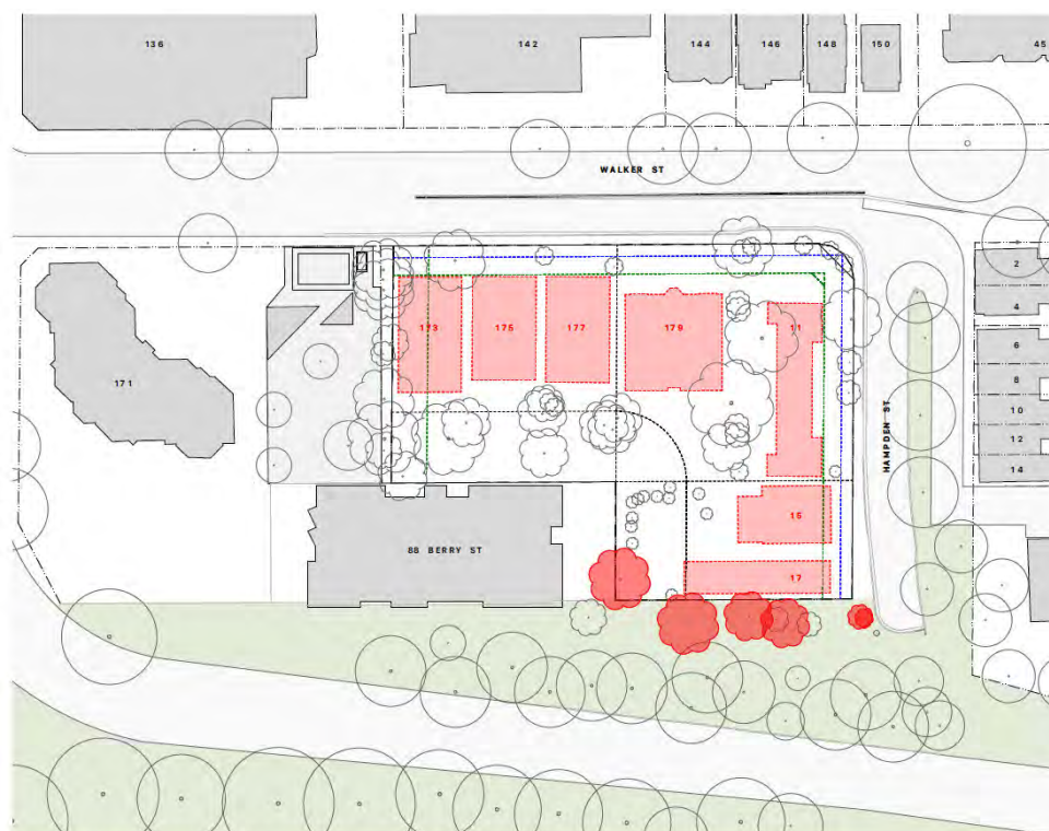
Figure 1: Demolition Plan (FJM Studios)
