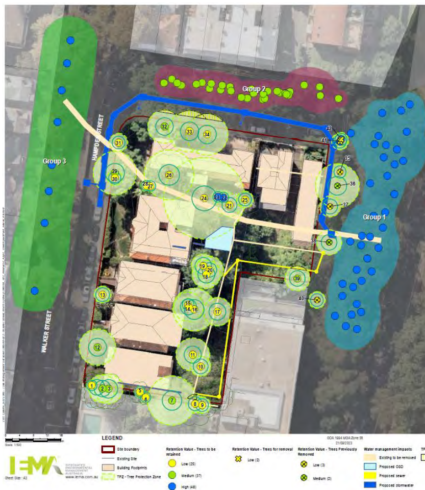
Figure 3: Extract of map showing trees to be retained on site, numbers in small circles, and those already removed or to be removed indicated by crosses in small circles (Tree Management Strategies).
