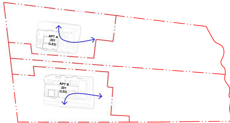
LEVEL R4-L03 - CROSS VENTILATION
