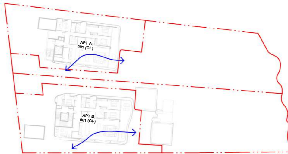
LEVEL R4 GROUND - CROSS VENTILATION (2/2)
