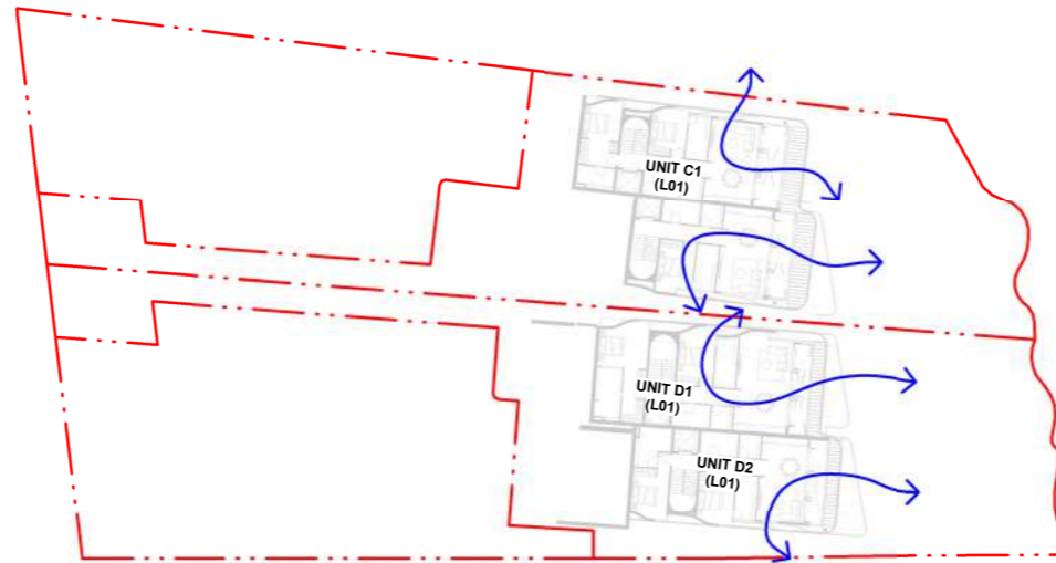
LEVEL R2-L01 - CROSS VENTILATION (4/4)
