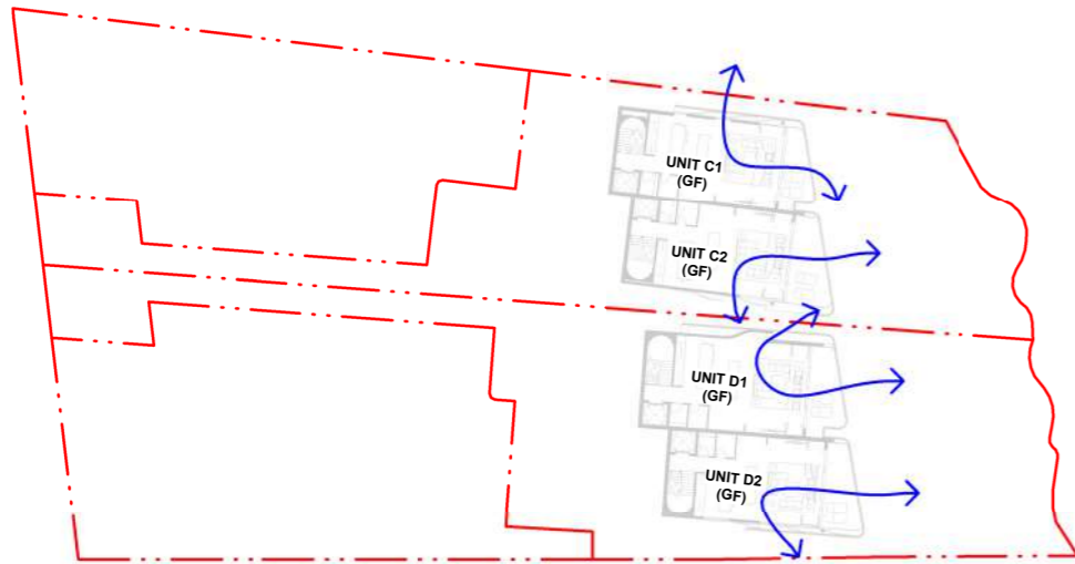
LEVEL R2-GROUND - CROSS VENTILATION (4/4)
