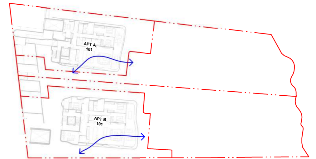
LEVEL R4-L01 - CROSS VENTILATION (2/2)
