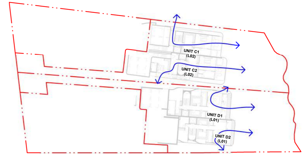
LEVEL R2-L02 - CROSS VENTILATION (4/4)
