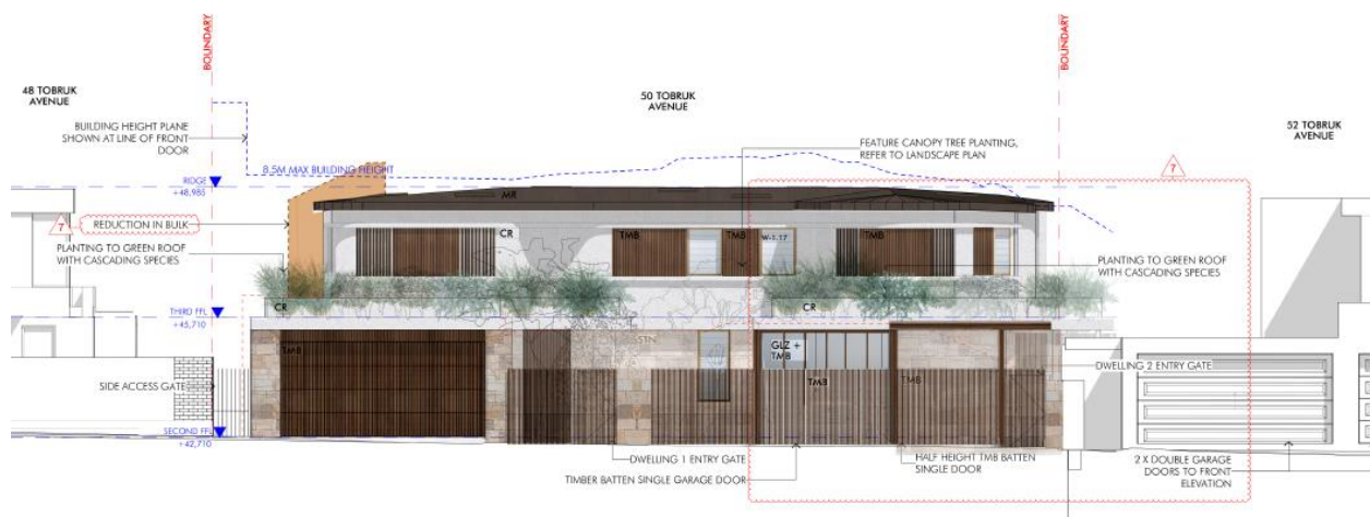
At street level the building is under the maximum building height (dotted blue line). The originally proposed lift tower has been removed (tan) to reduce bulk and height, and the façade adjusted to reduce visual impact and intrusiveness of parking structures, and reduce the symmetry of the original design (Arae Architecture).
