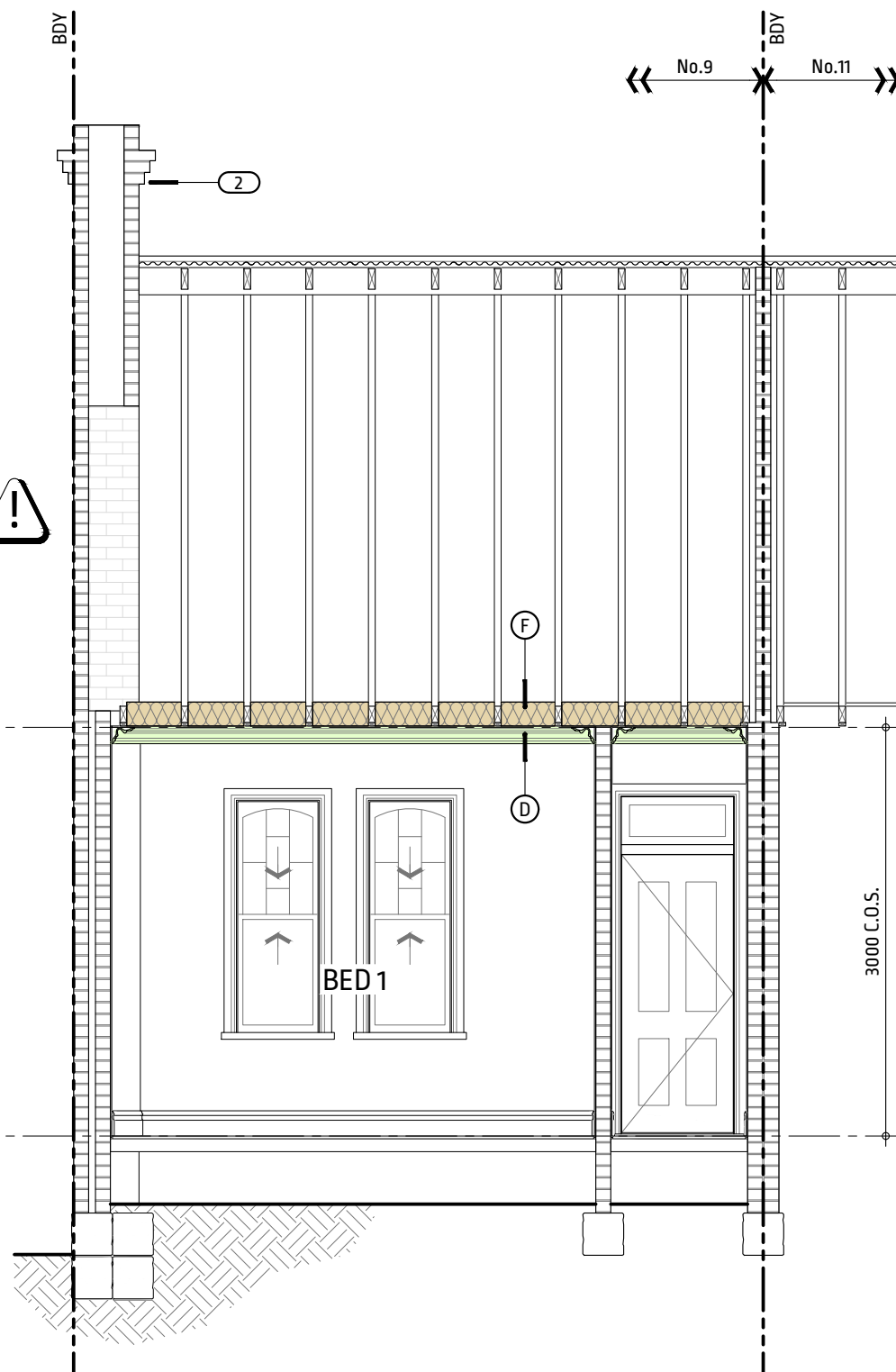
X1 PROPOSED CROSS SECTION X1 A100 SCALE 1:50
