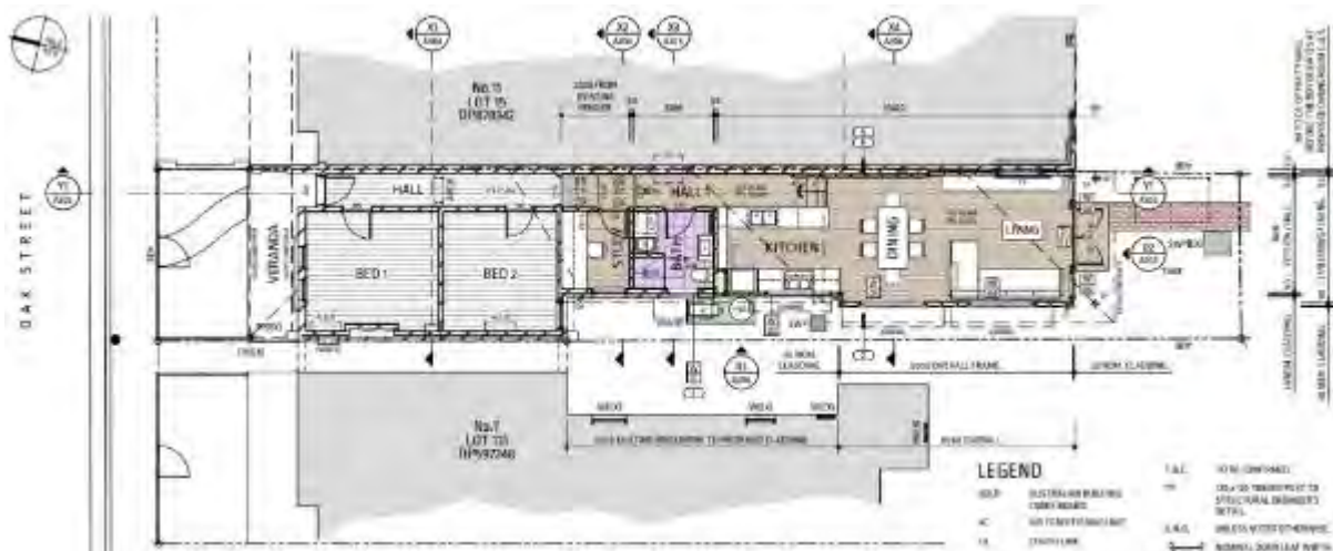
Figure 2: Proposed Ground Floor Plan
