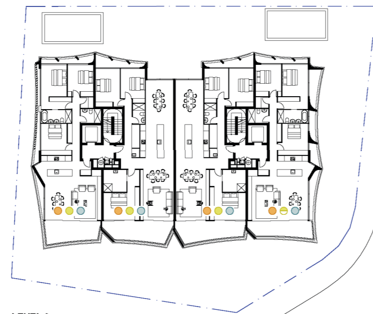
LEVEL 3 SOLAR & CROSS VENTILATION DIAGRAM
