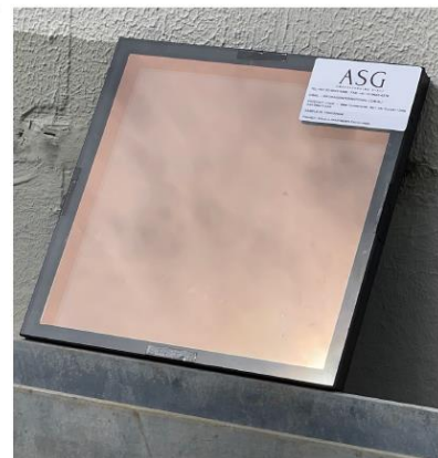
Tinted Glass: ASG Glass: 6mm Champagne 40-1 - 0n Clear + 12mm Argon + 6mm Clear Visible Light Transmission (VLT): 37% U-Value: 1.42 Solar Heat Gain Coefficient (SHGC): 0.23 External Reflectivity (ER): 10%
