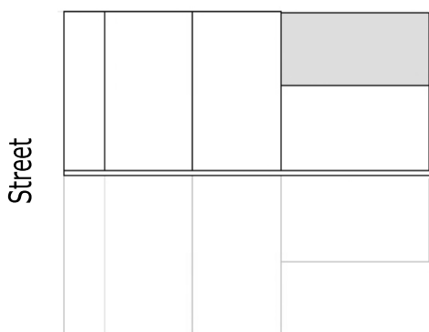
Figure B-13.47: Locate changes at the rear. Consider the impact on the attached pair, avoid changes that will affect common walls.
