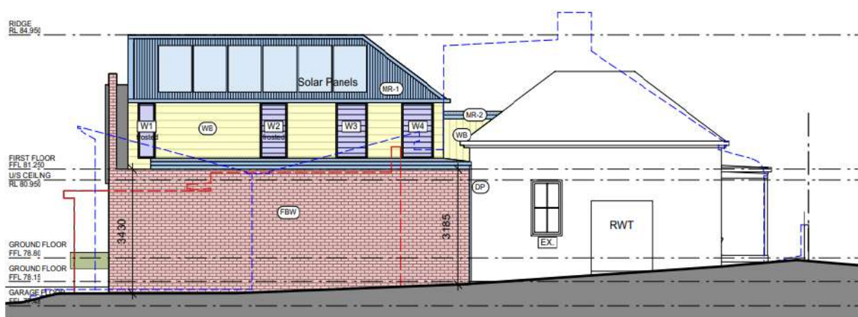
Figure 3 - West Elevation, DA07 Issue B
