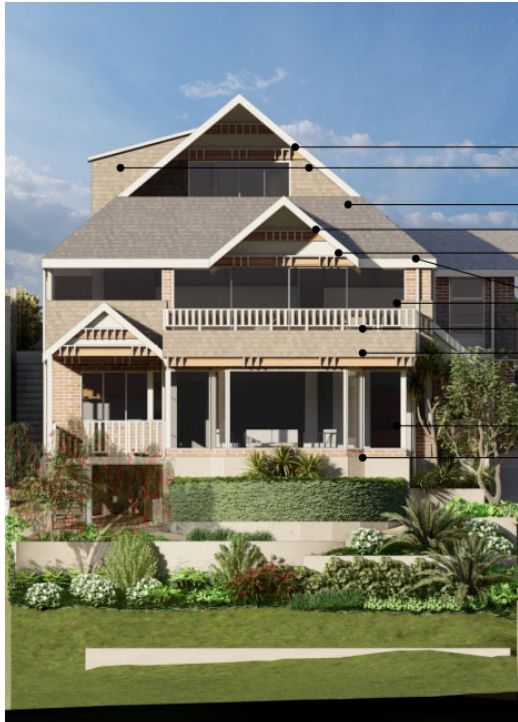
Figure 56 - Schedule of external finishes. Note the timber detailing to the balustrade as well as the timber brackets to the gable and verandahs. These details have been reconstructed based on existing building elements, see below.
