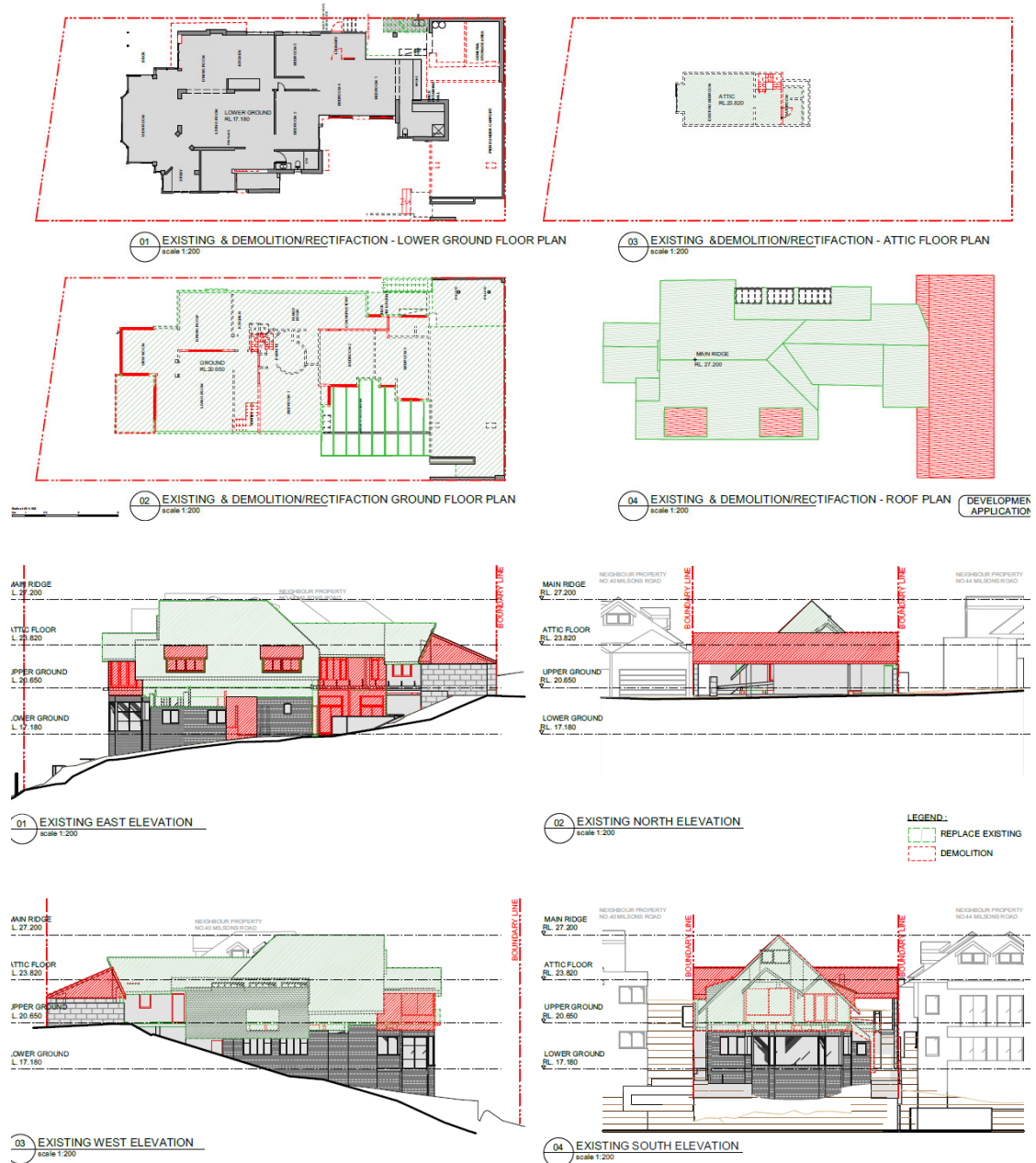
Figure 42 - These drawings identify those elements of the existing building proposed to be demolished (red hatch) and those areas to be replaced (green hatch). Those areas in grey are to be retained.
