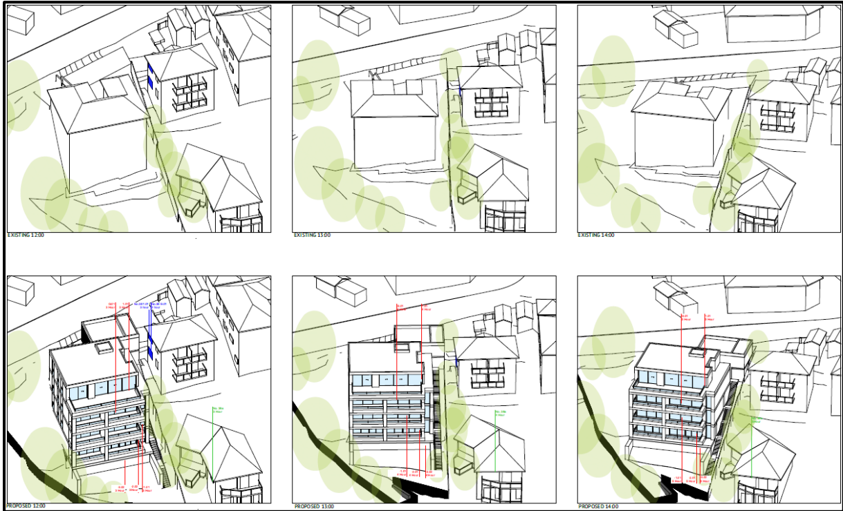
Figure 17: June 21, views from the sun - Existing (top) vs. Proposed (bottom) 12:00 pm, 1:00 pm and 2:00 pm (left to right)
